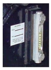
Figure 13. Hydraulic Oil Tank and Sight Gauge
