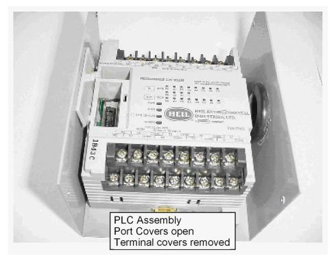
Various vehicle applications use the Mni PLC. These applications require two (2) Electronic Over Speeds (EOS). These applications generally use a tandem pump. The EOS set points are part of the PLC program, therefore you do not need the EOS screws.
