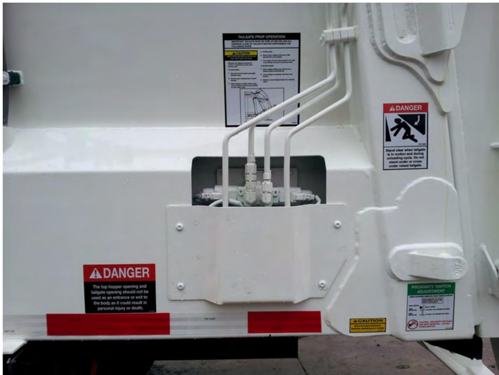
Figure 18. Rear Cover Protecting Electric-Over-Hydraulic Portion of Valve
