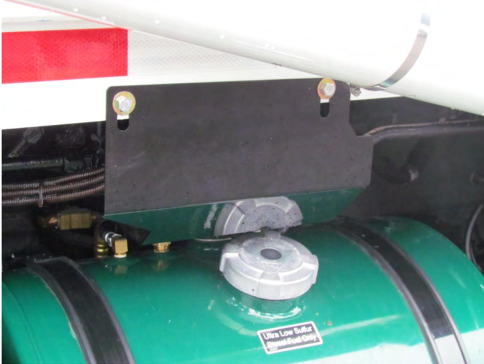
Figure 17. Steel Cover Protecting Arm, Fork and Packer Hydraulic Circuits
