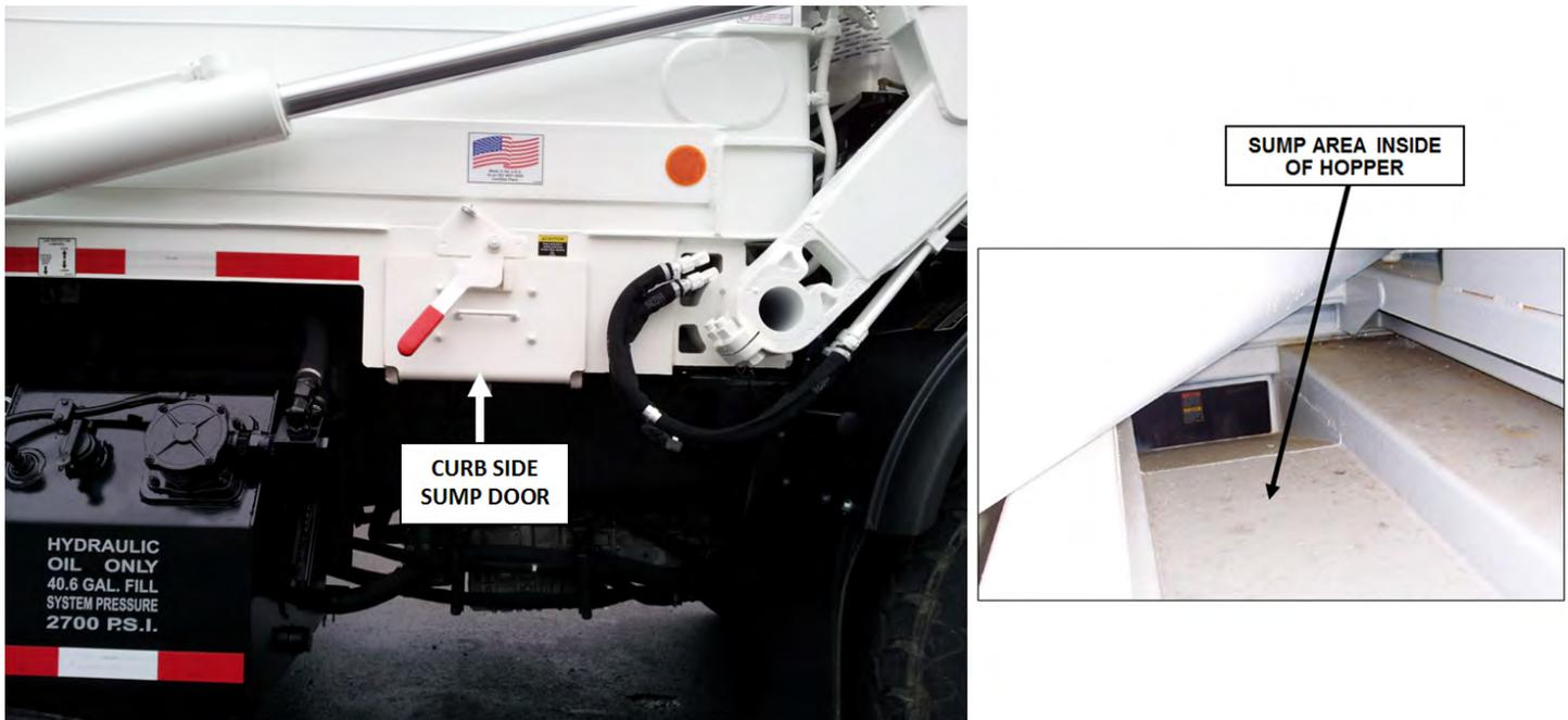
Figure 10. Sump Door and Internal Area
