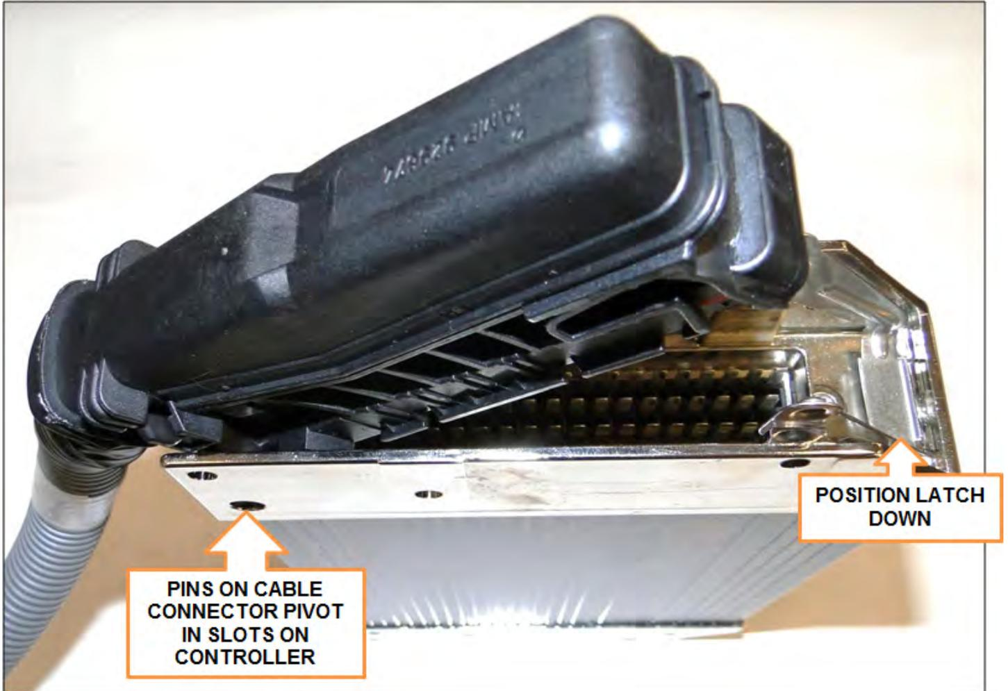
Figure 33. Cable Connector Pivoting on Controller
