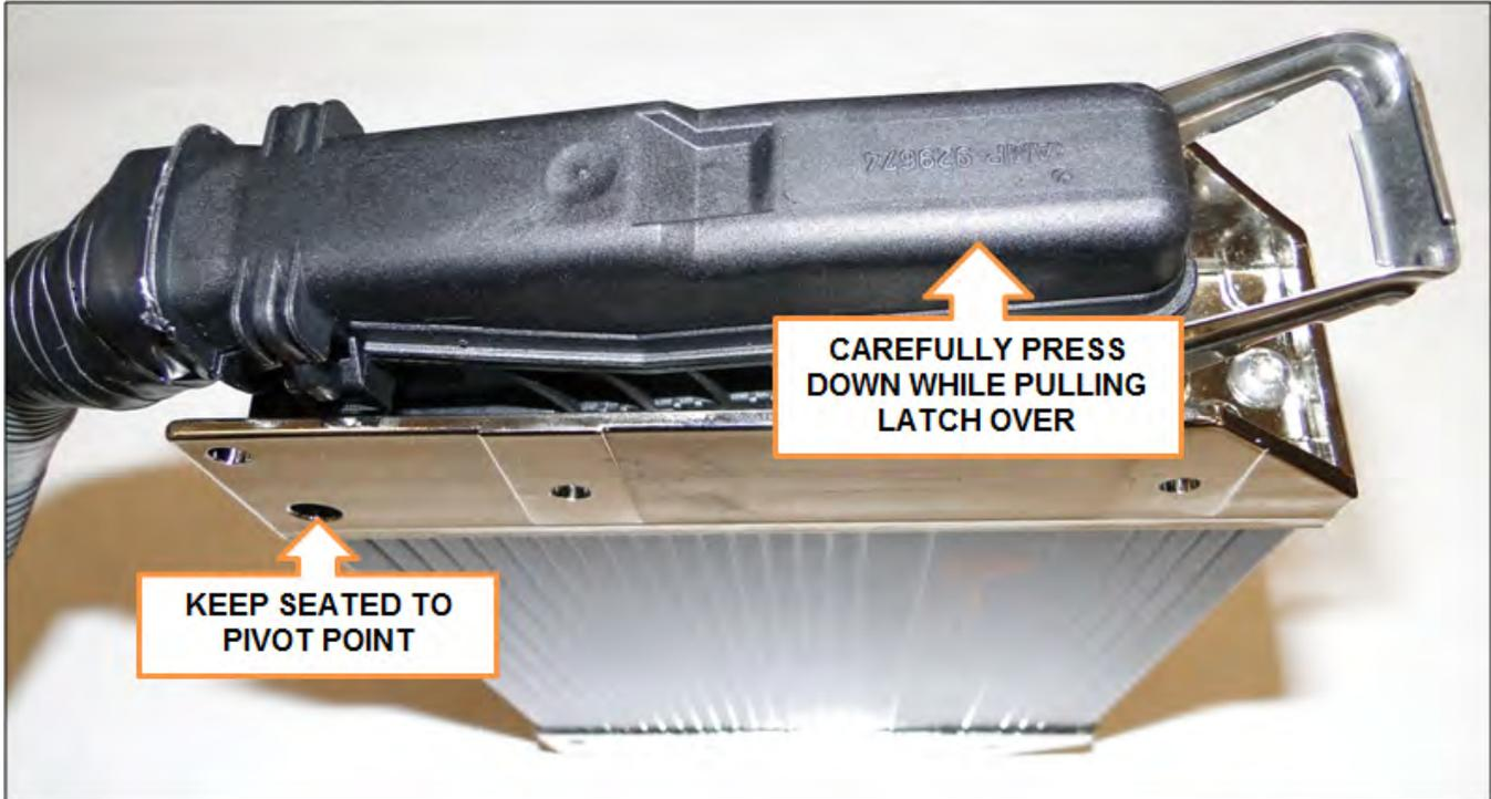
**Figure 34. Slowly Press Down While Keeping Left Cable Connector Pivot Point in Place**
