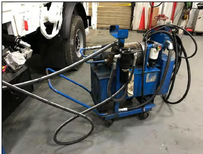
Figure 23. Auxiliary Hydraulic Supply Unit
