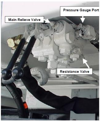
Figure 11. Underbody Valve: Main Relief Valve, Pressure Gauge Port and Resistance Valve
