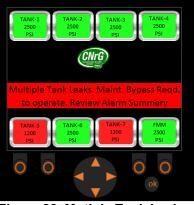
Figure 82. Mutiple Tank Leaks. Maintenance Bypass Required.
