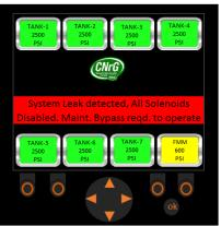
Figure 83. System Leak. Maintenance Bypass Required.
