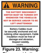
Figure 23. Warning: Disconnect battery, PN 212-2875
