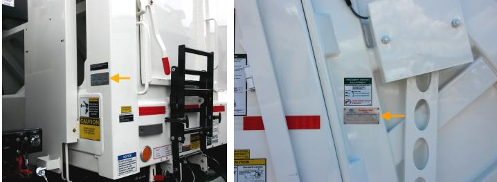
Figure 2. Body Serial Plate
