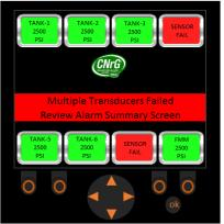
Figure 78. Multiple Pressure Transducer Sensors Unplugged/Faulty
