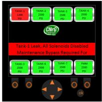
Figure 81. Tank 1 Leak. Maintenance Bypass Required.
