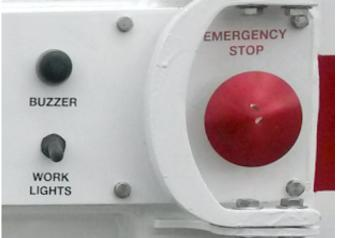
Figure 55. Outside Tailgate Controls (Both Sides)
