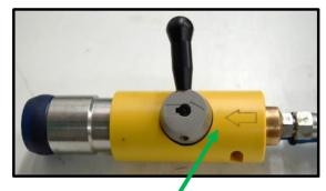
\*\*\*NOTE: Arrows must be aligned as shown to allow proper engagement of the hose with the fill receptacle.
