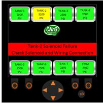
Figure 96. Display Screenshot: Tank 2 Solenoid Failure
