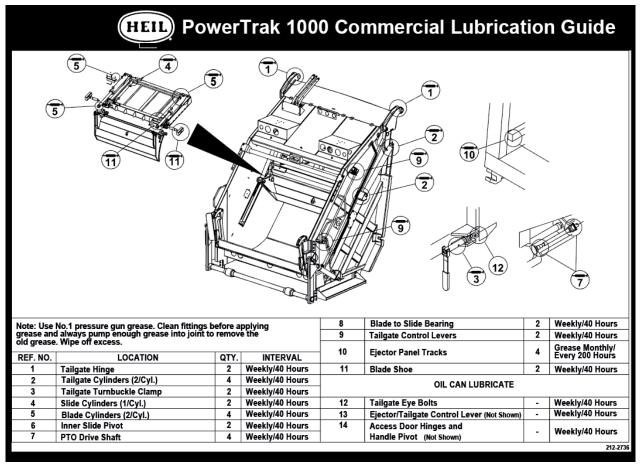
Figure 39. Lubrication Guide, PN 212-2736
