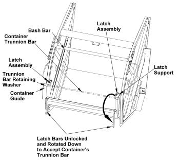
Figure 71. Latch Bars Rotated Down
