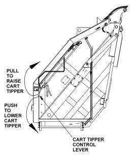
Figure 68. Cart Tipper Control Lever
