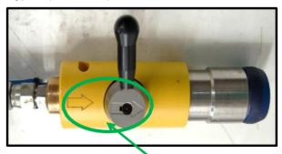
Arrows must be aligned and pointing toward the fill receptacle to allow fueling.
