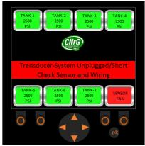
Figure 89. Pressure Transducer Sensor behind FMM Unplugged/Faulty
