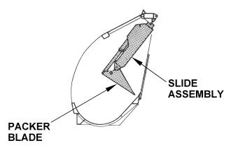
Figure 59. Packer Blade Starting Position
