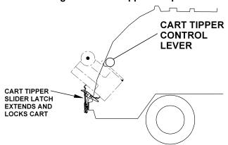
Figure 70. Loading Refuse with Cart Tipper
