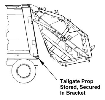
Figure 54. Open Tailgate for Tailgate Props
