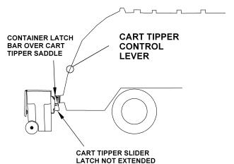
Figure 69. Cart Tipper Setup
