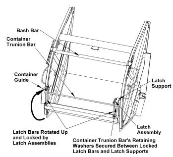
Figure 72. Latch Bars Rotated Up
