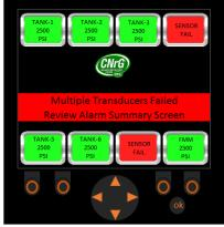
Figure 90. Multiple Pressure Transducer Sensors Unplugged/Faulty
