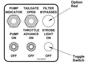
**Figure 45. Control Panel Optional Functions**
