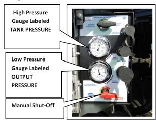
Figure 76. Manual Shut-Off Valve
