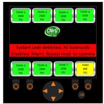
Figure 95. System Leak. Maintenance Bypass Required.
