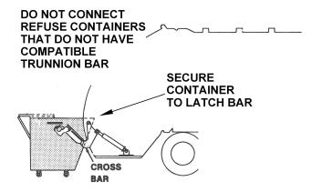
Figure 64. Arm Mechanism Setup
