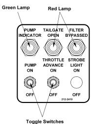
Figure 44. Control Panel Standard Functions
