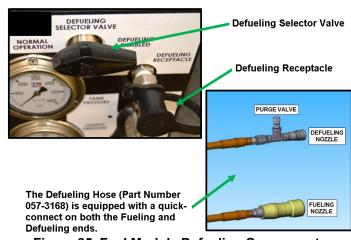
Figure 85. Fuel Module Defueling Components
