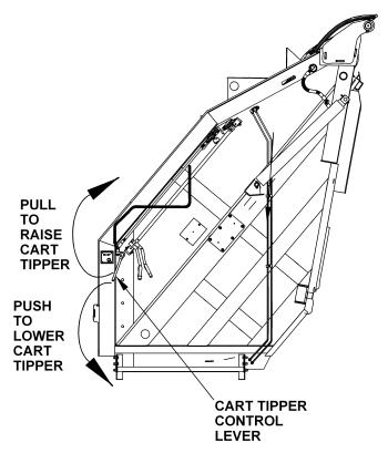
Figure 51. Cart Tipper Control Lever
