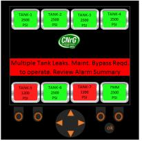
Figure 94. Mutiple Tank Leaks. Maintenance Bypass Required.
