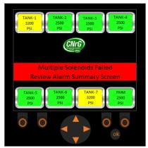
Figure 97. Display Screenshot: Multiple Solenoids Failed
