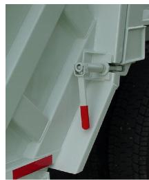
Figure 53. Tailgate Clamps (Turnbuckles)
