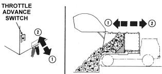
1. PULL EJECTOR LEVER TO EXTEND EJECTOR PANEL AND DUMP REFUSE
