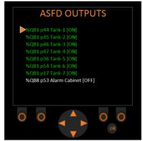
Figure 102. Display Screenshot: System Outputs
