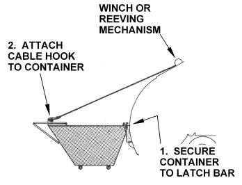
Figure 62. Reeving Mechanism or Winch Setup
