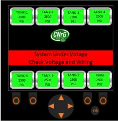
Figure 105. Display Screenshot: System Under Voltage
