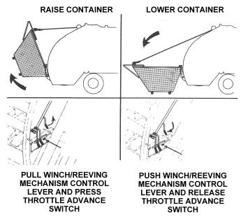
Figure 63. Loading Refuse with Reeving Mechanism or Winch
