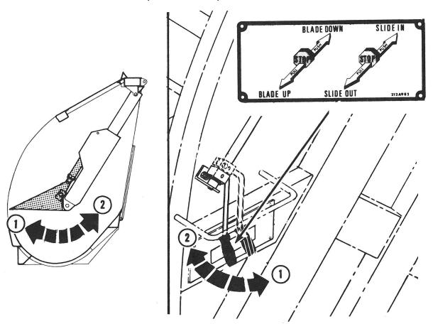
Figure 46. Packer Blade Control Lever
