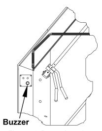
Figure 49. Buzzer Location
