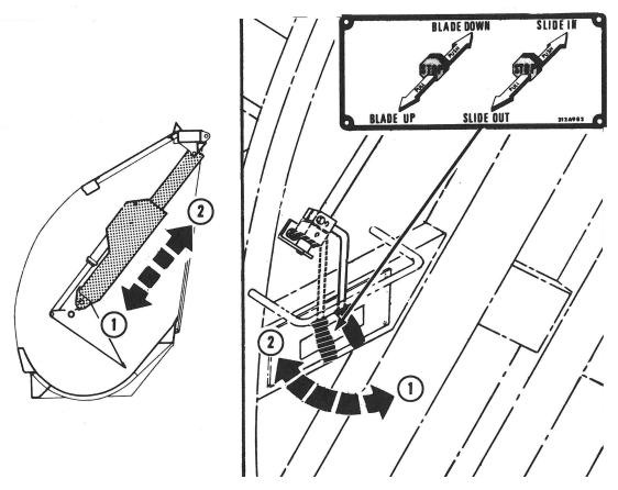
Figure 47. Slide Control Lever
