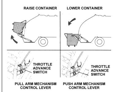
Figure 65. Loading Refuse with Arm Mechanism
