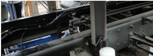
Figure 60. Lower Body onto Factory Body Props
