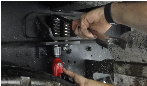
Figure 57. Removing Bolts and Springs from Chassis Mounting Brackets
