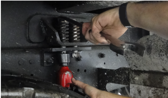
Figure 55. Removing Bolts and Springs from Chassis Mounting Brackets
