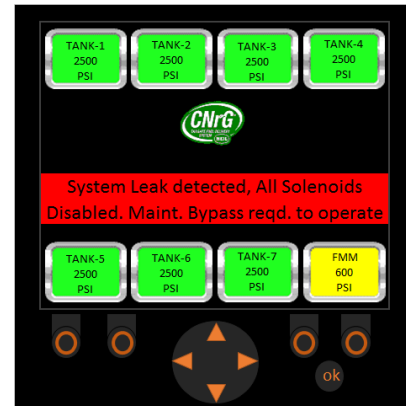
Figure 106. System Leak. Maintenance Bypass Required.
