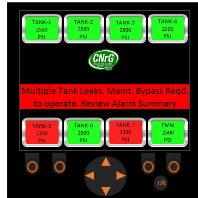
Figure 105. Multiple Tank Leaks. Maintenance Bypass Required.
