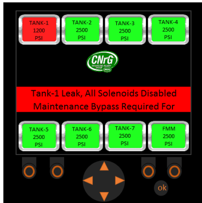
Figure 104. Tank 1 Leak. Maintenance Bypass Required.
