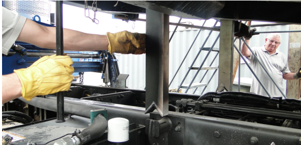
Figure 59. Release and Lower Factory Body Props
