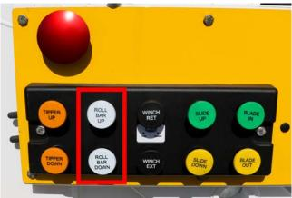
Figure 40. Tailgate Optional Roll Bar Push Button Controls (Red Outline)
