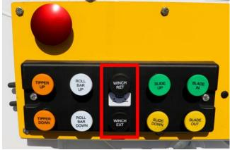
Figure 41. Tailgate Optional Winch Push Button Controls (Red Outline)
