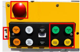
Figure 33. Tailgate Standard Outside Push Button Controls (Red Outlines)
