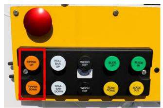
Figure 39. Tailgate Optional Tipper Push Button Controls (Red Outline)
