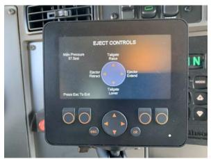
Figure 47. In-Cab Control Tailgate and Ejection Controls
