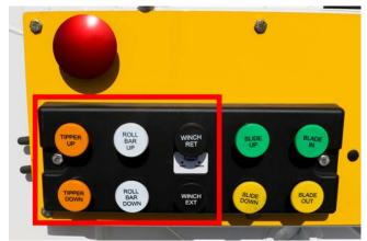
Figure 38. Tailgate Optional Equipment Push Button Controls (Red Outline)
