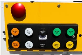
Figure 32. Tailgate Push Button Control Panel
