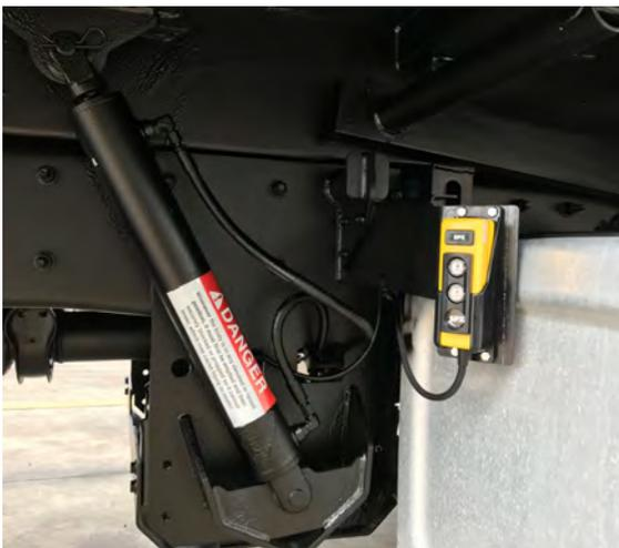
Figure 10. Typical Service Hoist Controls Location
