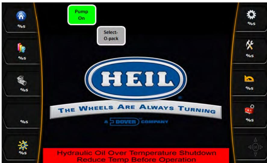
Indication: A. Hydraulic Oil over temperature shutdown.
