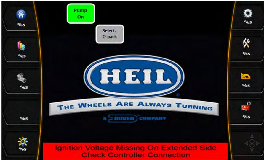
Indication: A. No Ignition Voltage on Extended side controller.
