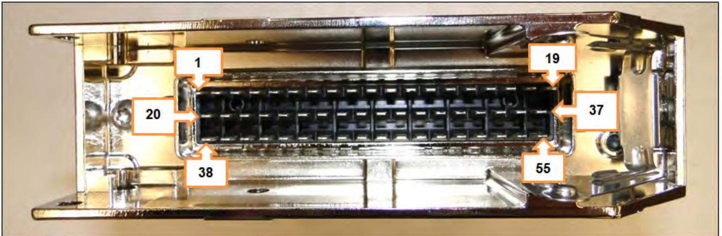
**Figure 26. Controller Pin Number Locations (For 80 I/O, Same for Both Controller Sides)**
