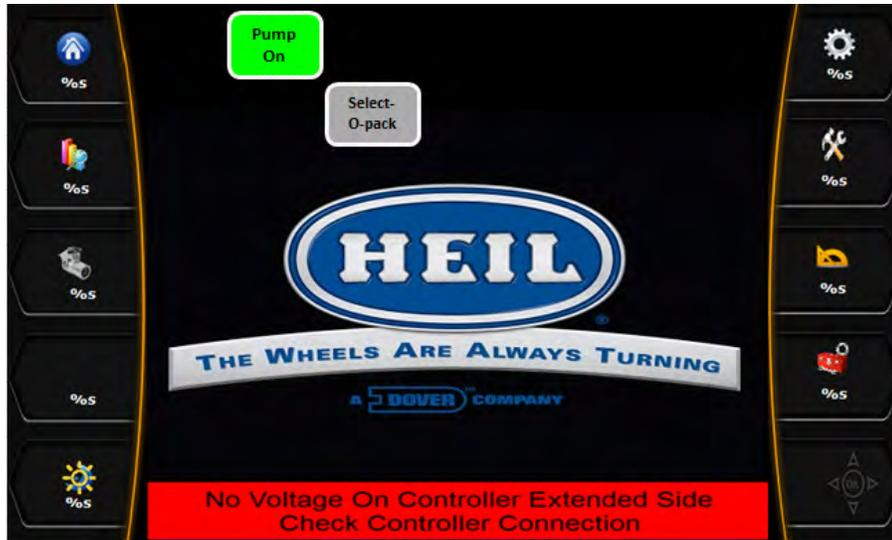
Indication: A. No Voltage on Extended side controller.
