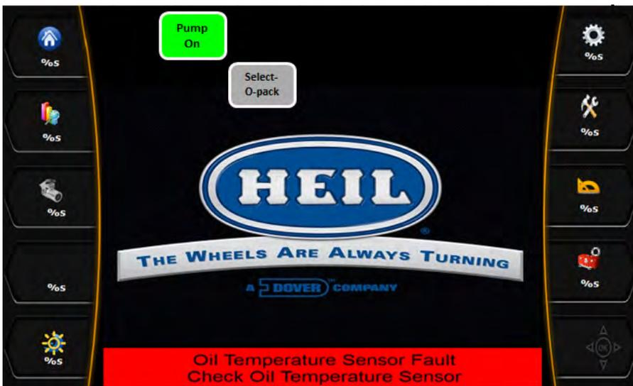
Indication: Oil Temperature Sensor fault
