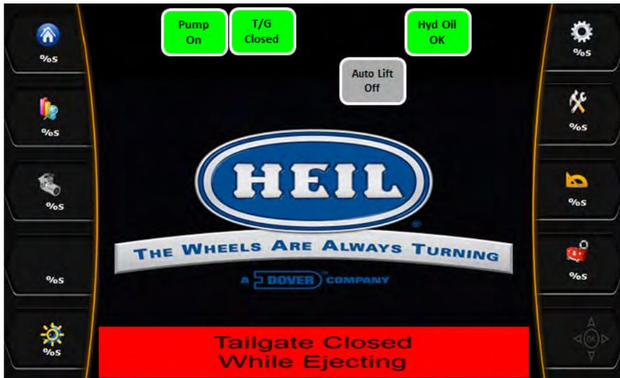
Indications: Packer Fully Extended and Tailgate Closed inputs are lit.
