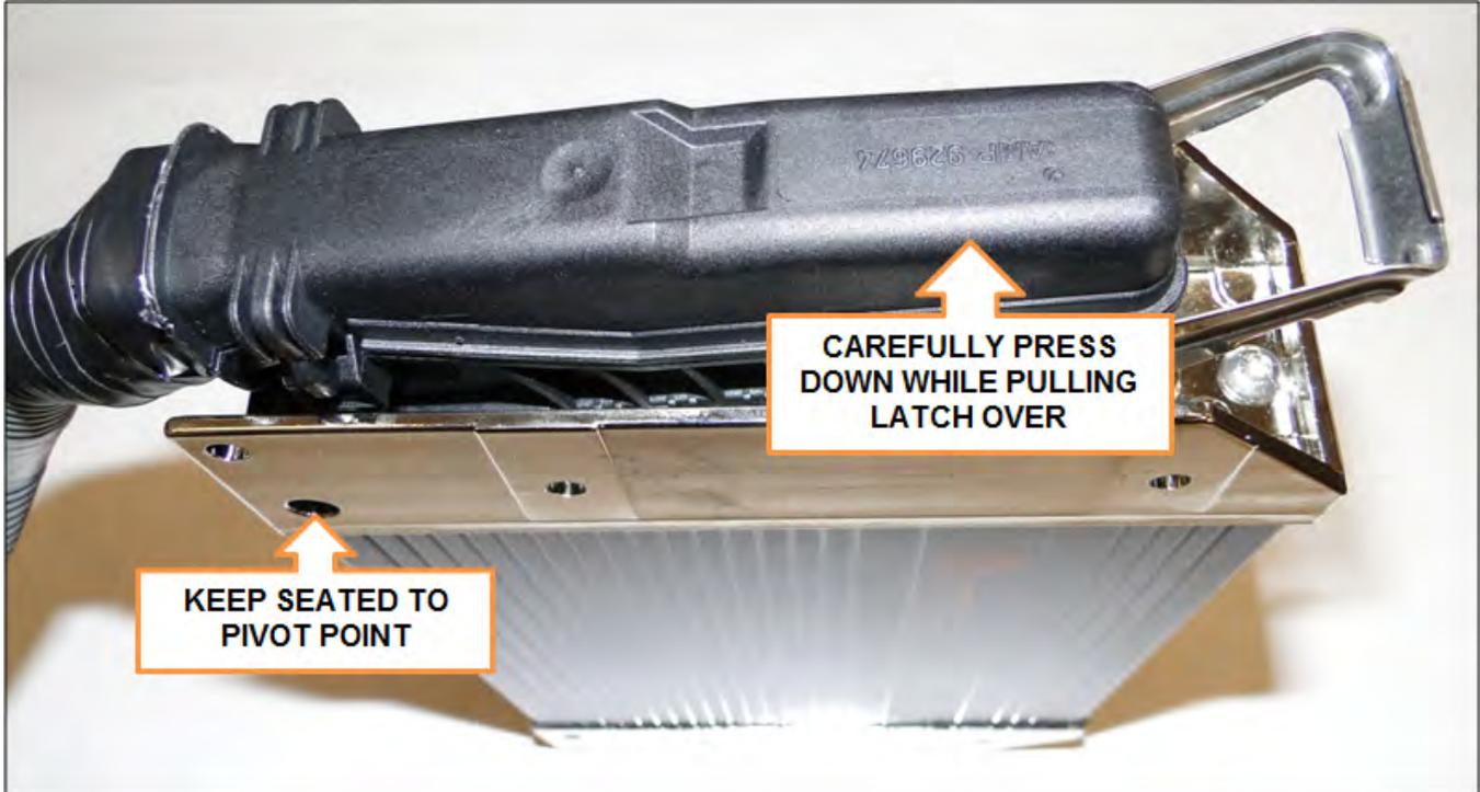
**Figure 30. Slowly Press Down While Keeping Left Cable Connector Pivot Point in Place**
