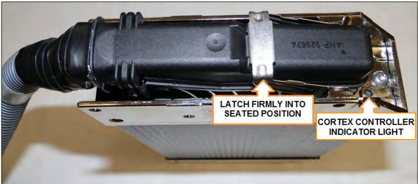
**Figure 31. Latch Controller to Cable Connector**
