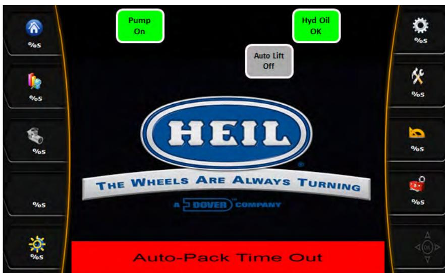
Indications: Diagnostic message will be displayed in the Insight display. Packer extend prox. is not activated 35 seconds after start of extend cycle.
