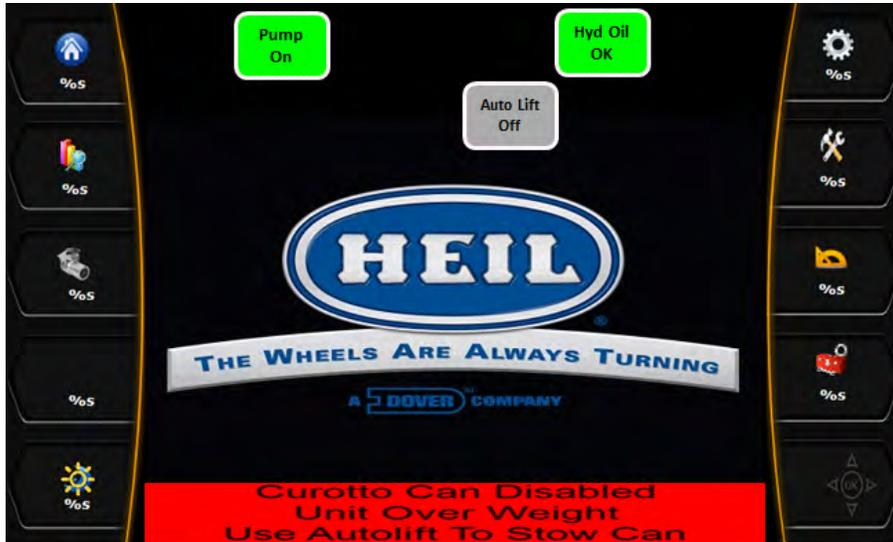
Indication: A. Scale Alarm-2 ON due to Overweight.
