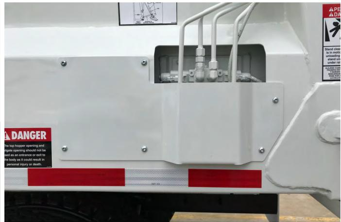
Figure 19. Tailgate Valve with Cover
