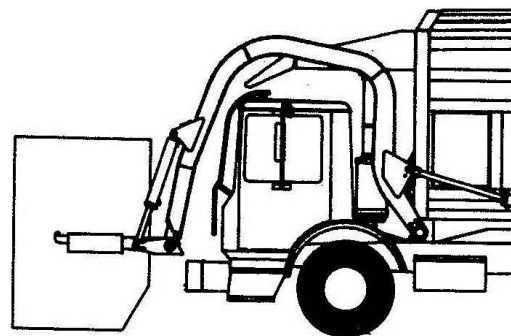
Figure 81. Rotate Container Back before Lowering
