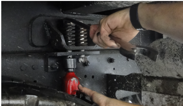
Figure 65. Removing Bolts and Springs from Chassis Mounting Brackets
