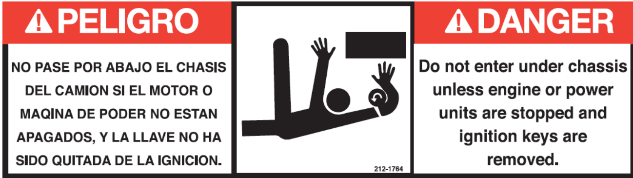
Figure 13. Danger: Do Not Enter Under Chassis, PN 212-1764
