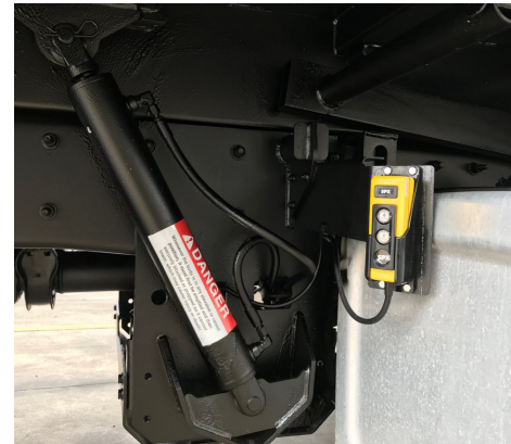
Figure 62. Typical Service Hoist Controls Location
