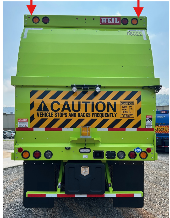
Figure 9. CNrG Tailgate PRD Vents Location (Top of Tailgate, Red Arrows)
