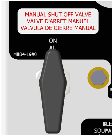
Figure 23. FMM Manual Shut Off Valve
