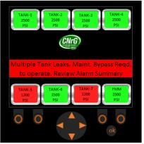
Figure 71. Mutiple Tank Leaks. Maintenance Bypass Required.
