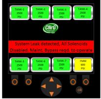
Figure 72. System Leak. Maintenance Bypass Required.
