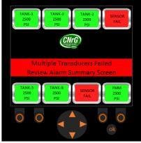
Figure 67. Multiple Pressure Transducer Sensors Unplugged/Faulty
