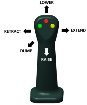
Figure 41. Joystick Movements/Functions
