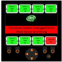
Figure 66. Pressure Transducer Sensor behind FMM Unplugged/Faulty
