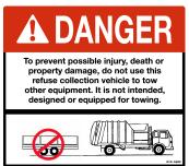
Figure 19. Danger: Do not use for towing, PN 212-1820
