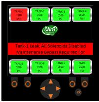
Figure 70. Tank 1 Leak.
