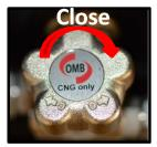
Figure 63. Cylinder Manual Shut-Off Valve
