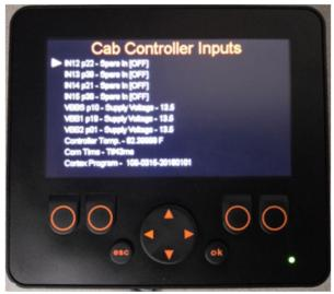
Figure 37. Cab Controller Inputs
