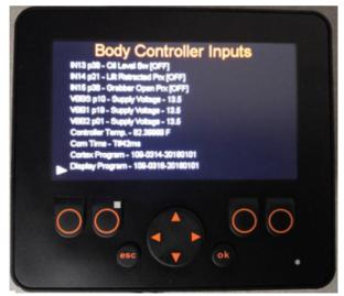
Figure 36. Body Controller Inputs
