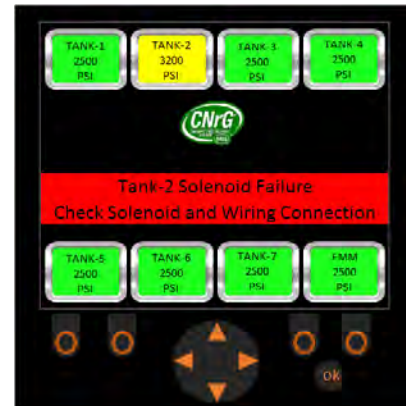
Figure 89. Display Screenshot: Tank 2 Solenoid Failure
