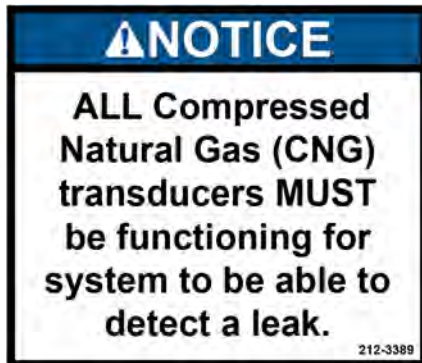
Figure 76. Notice, CNrG Solenoid System, Transducers MUST be functioning, PN 212-3389
