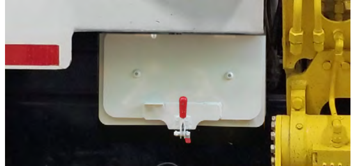
Figure 51. Curb Side Hopper Sump Door Closed
