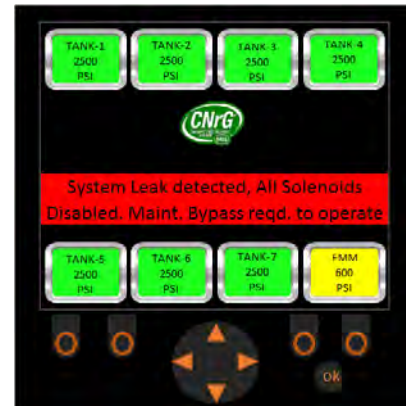
Figure 88. System Leak. Maintenance Bypass Required.
