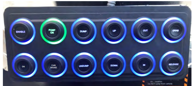
Figure 41. Manual Control Push Button Controls (DISABLE and PUMP OFF buttons shown may not be found on all units.)
