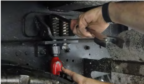
Figure 44. Removing Bolts and Springs from Chassis Mounting Brackets
