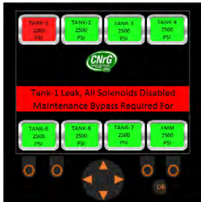
Figure 86. Tank 1 Leak. Maintenance Bypass Required.
