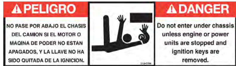
Figure 11. Danger: Do not enter under chassis, PN 212-1764
