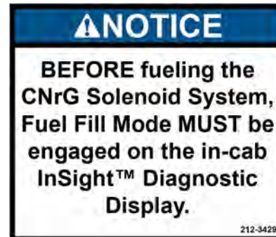
Figure 77. Notice, CNrG Solenoid System, Fuel Fill Mode MUST Be Engaged, PN 212-3429
