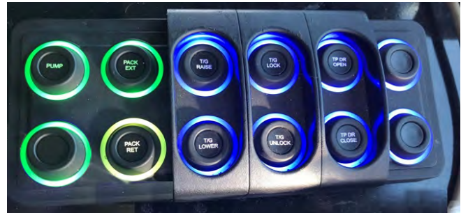
Figure 39. Main Push Button Controls
