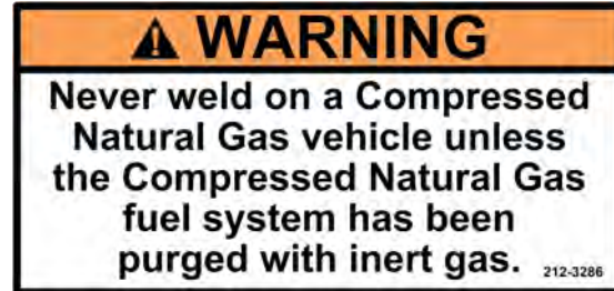
Figure 71. Warning, Never weld on CNG vehicle unless purged, PN 212-3286
