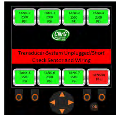
Figure 82. Pressure Transducer Sensor behind FMM Unplugged/Faulty
