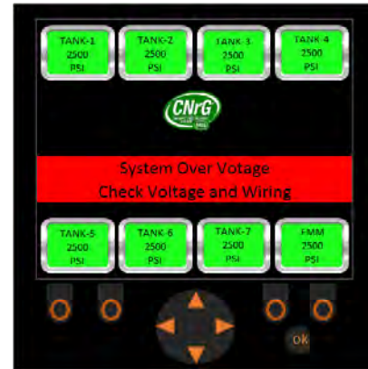
Figure 97. Display Screenshot: System Over Voltage
