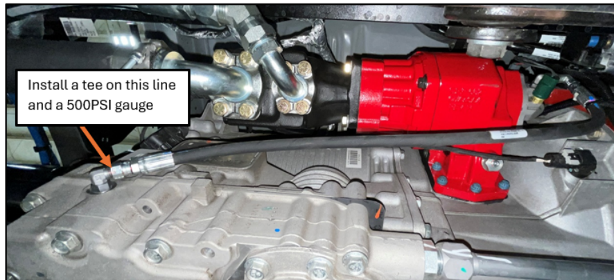
Figure 14. Transmission Pressure Feed to PTO.
