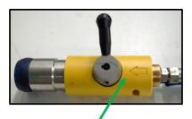
\*\*\*NOTE: Arrows must be aligned as shown to allow proper engagement of the hose with the fill receptacle.
