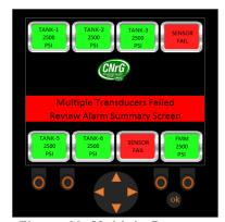
Figure 89. Multiple Pressure Transducer Sensors Unplugged/Faulty
