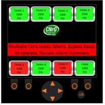
Figure 93. Mutiple Tank Leaks. Maintenance Bypass Required.
