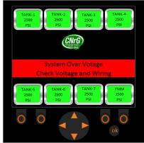
Figure 103. Display Screenshot: System Over Voltage
