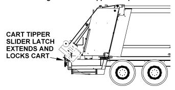
Figure 70. Loading Refuse with Cart Tipper
