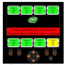
Figure 94. System Leak. Maintenance Bypass Required.
