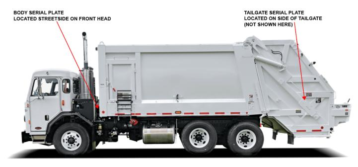
Figure 2. Serial Plate Locations.
