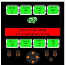
Figure 104. Display Screenshot: System Under Voltage
