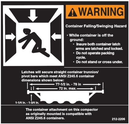
Figure 38. Warning: Container falling/swinging hazard, PN 212-2206
