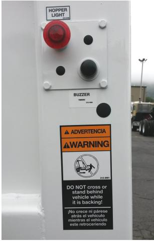
Figure 50. Buzzer and Hopper Light Switch Location
