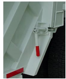
Figure 55. Tailgate Clamps (Turnbuckles)
