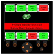
Figure 116. Multiple Pressure Transducer Sensors Unplugged/Faulty
