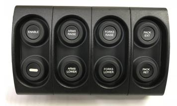
Figure 57. Optional Outside Curotto-Can Controls
