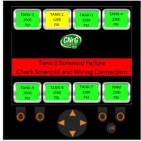
Figure 122. Display Screenshot: Tank 2 Solenoid
