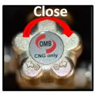
Figure 96. Cylinder Manual Shut-Off Valve
