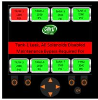
Figure 119. Tank 1 Leak. Maintenance Bypass Required.
