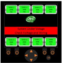
Figure 131. Display Screenshot: System Under Voltage
