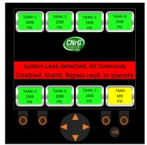
Figure 121. System Leak. Maintenance Bypass Required.
