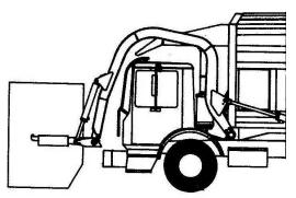
Figure 81. Rotate Container Back before Lowering
