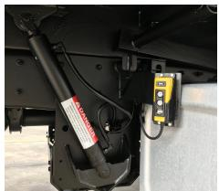
Figure 62. Typical Service Hoist Controls Location
