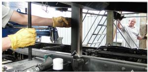
Figure 67. Release and Lower Factory Body Props
