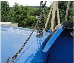
Figure 66. Front Body Chain Hook Lugs
