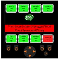
Figure 115. Pressure Transducer Sensor behind FMM Unplugged/Faulty
