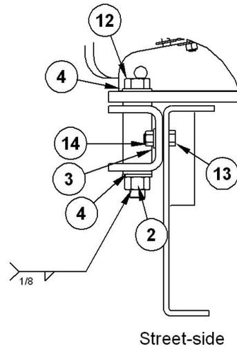
**Figure 15. Lift Mount Bolt Location**
