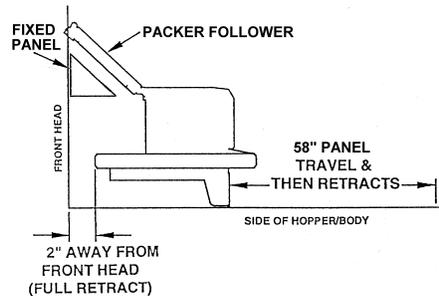
**Figure 38. Packer Pressure Panel Adjustment**
