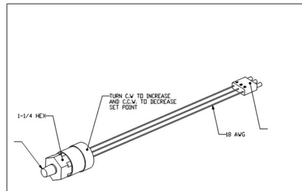
Figure 37. Packer Pressure Switch Adjustment
