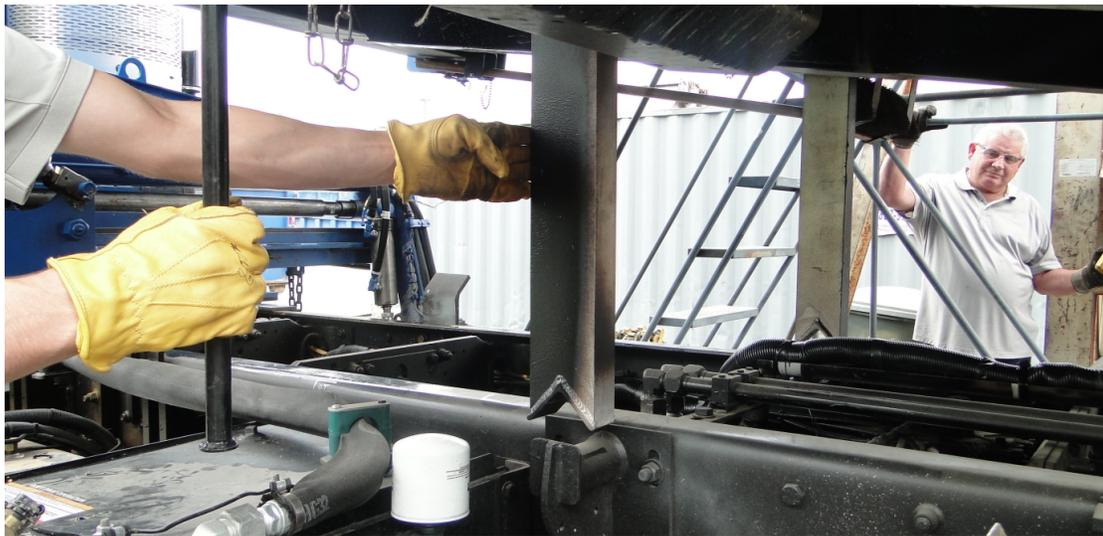
**Figure 30. Release and Lower Factory Body Props**
