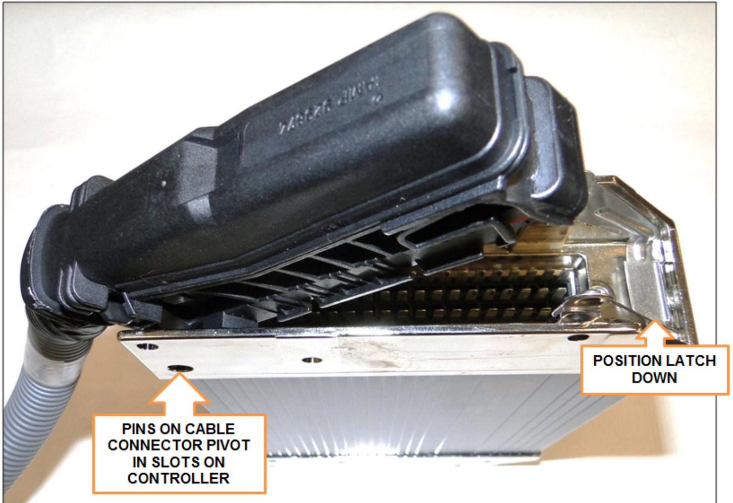
Figure 47. Cable Connector Pivoting on Controller
