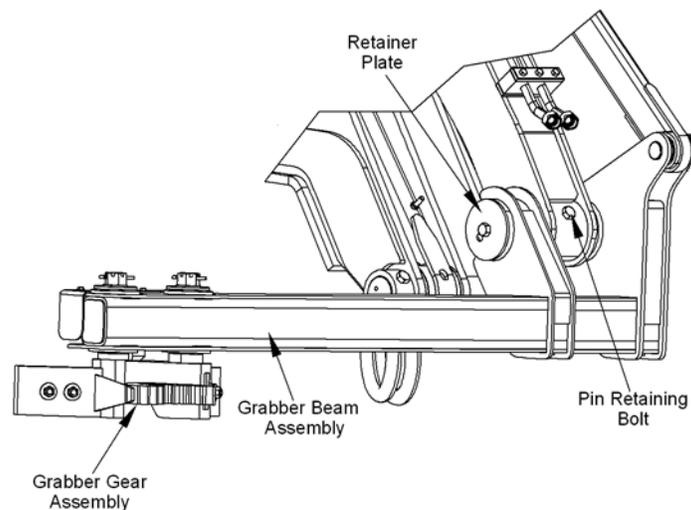
**Figure 23. Grabber Beam and Gear Assemblies with Retainer Plate and Pin Retaining Bolt**
