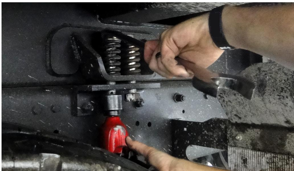
**Figure 26. Removing Bolts and Springs from Chassis Mounting Brackets**
