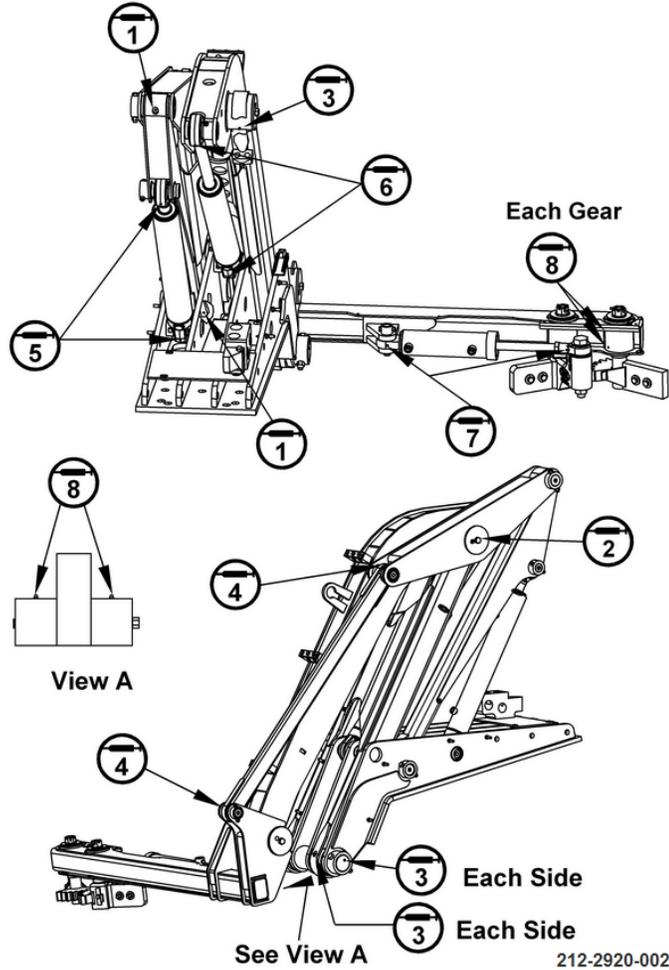
Figure 11. Python Lift Lubrication Guide
