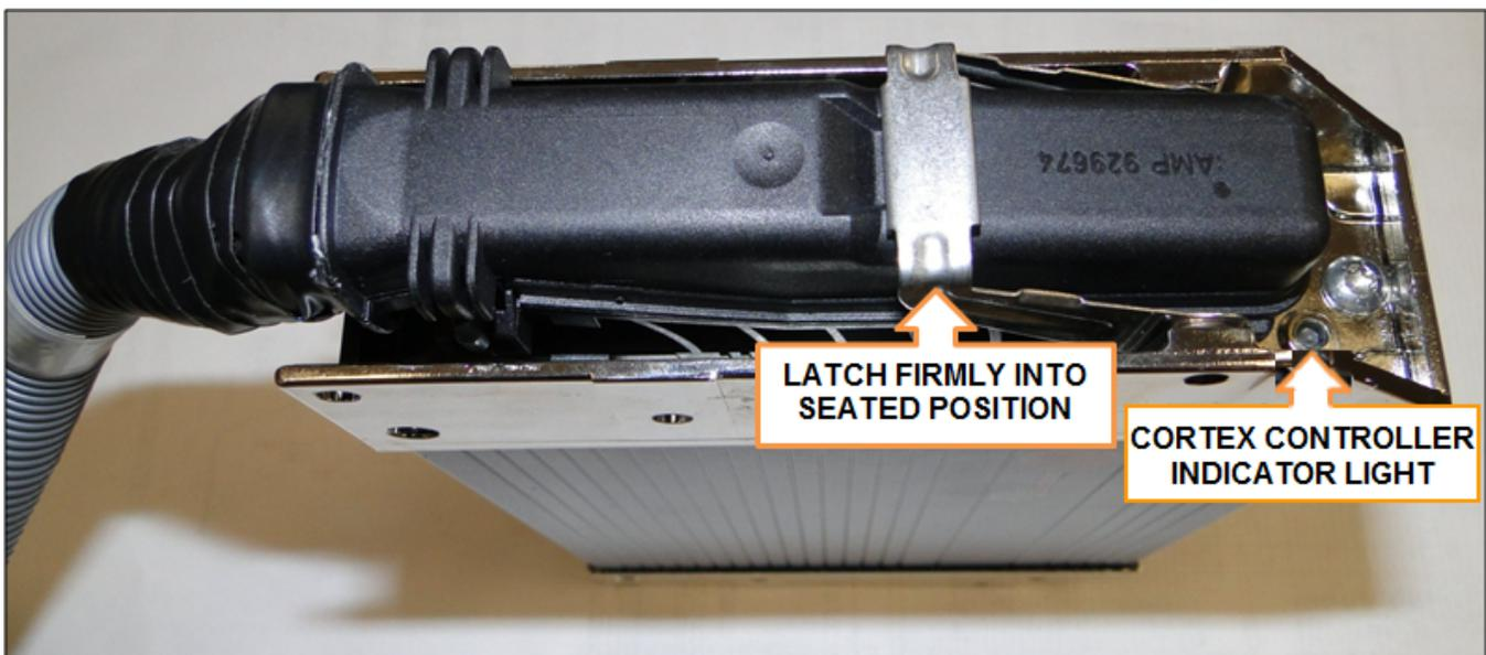
**Figure 49. Latch Controller to Cable Connector**
