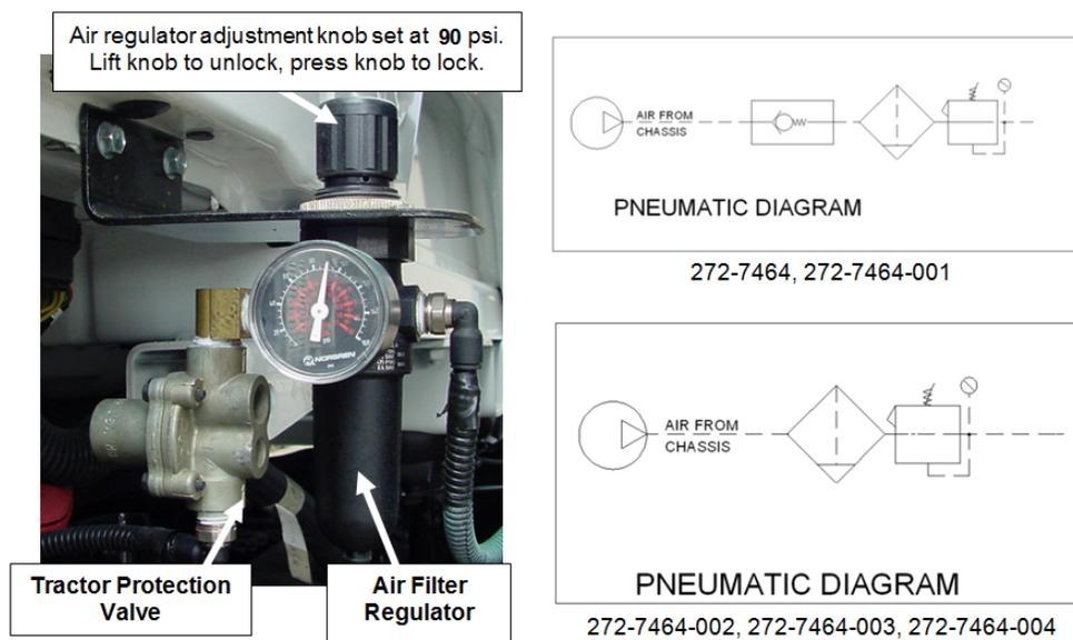
Figure 35. Air Supply Regulator
