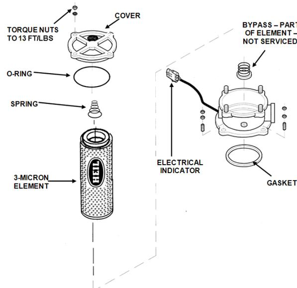
Figure 41. Hydraulic Oil Filter
