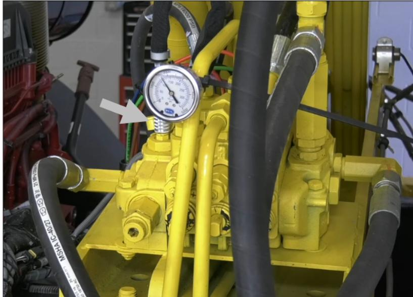
Figure 21. Inlet Section Pressure Gauge Port
