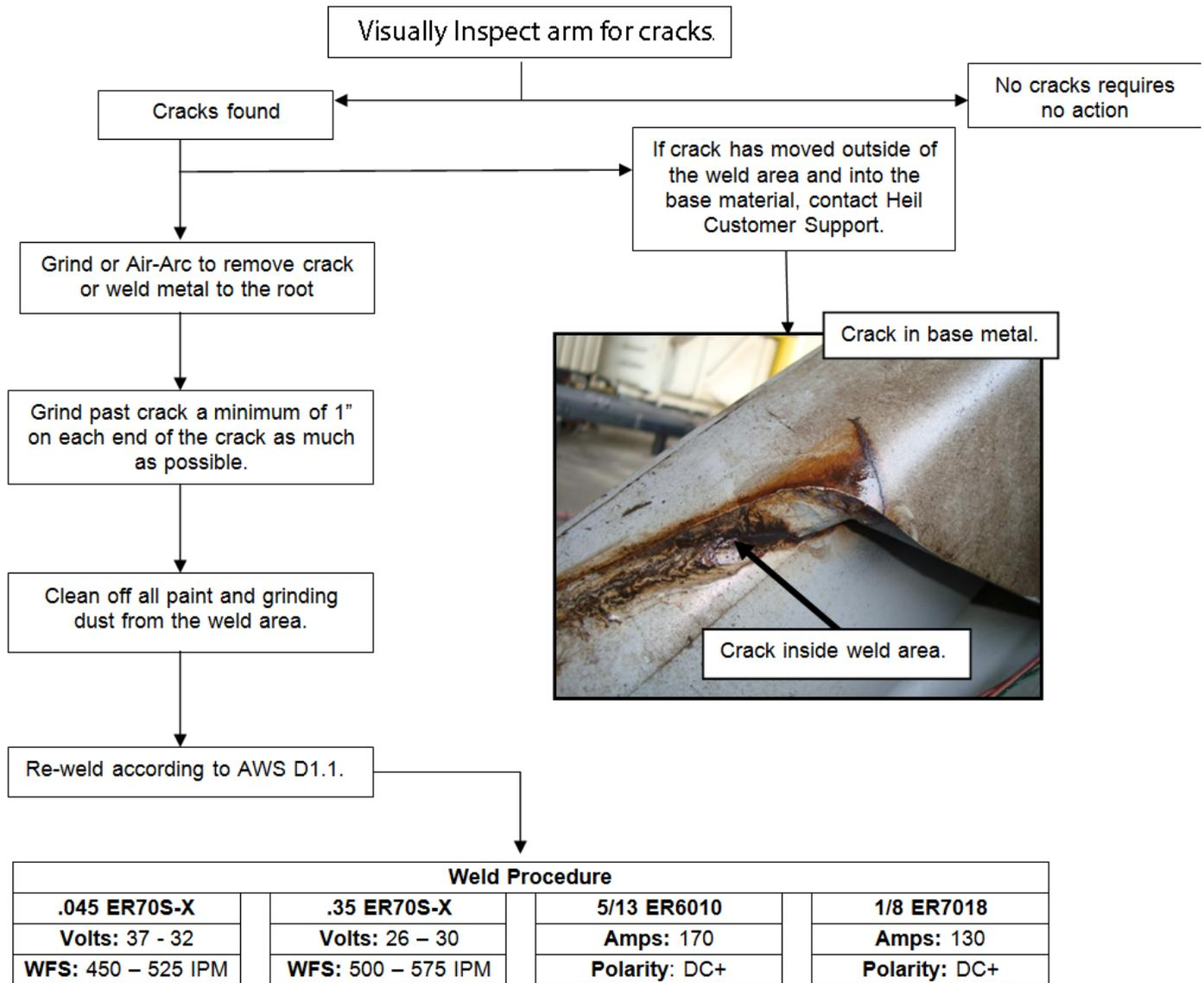
Follow these welding requirements for repairing the lift arm.
