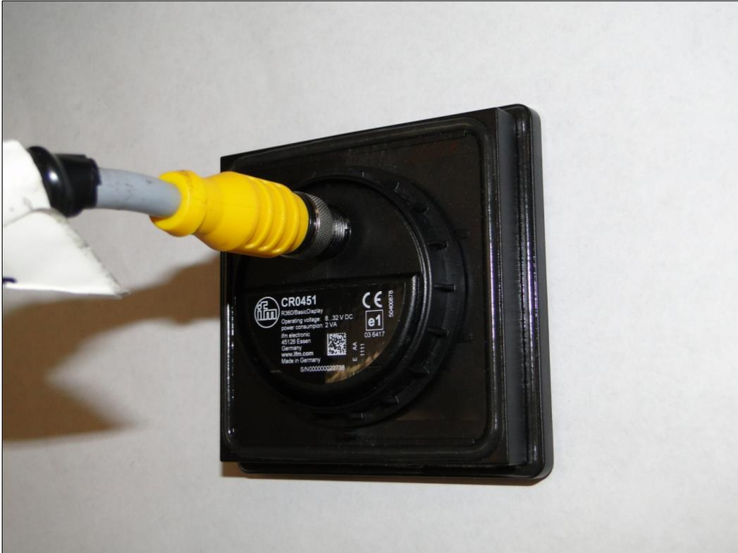
Figure 53. Rear View of Display with Cable Connected
