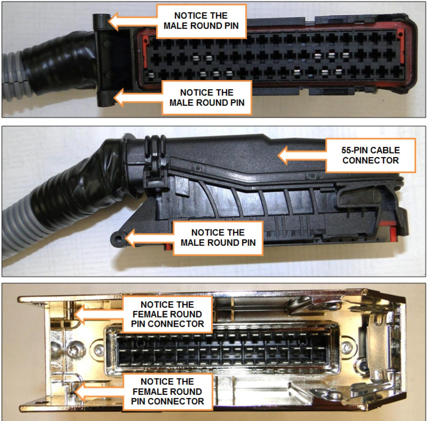
Figure 45. Cable Controller Plastic Male Hinge Pins and Controller Female Slot Connectors
