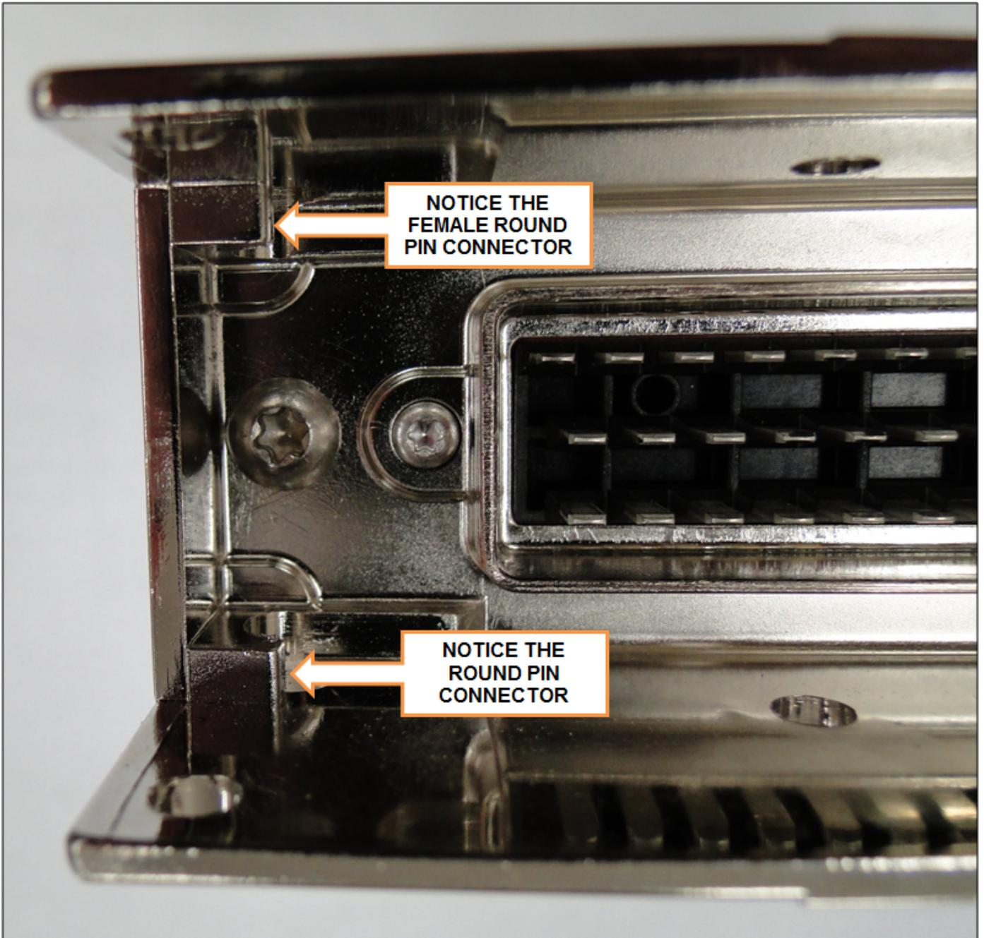
Figure 46. Female Controller Connector Slots
