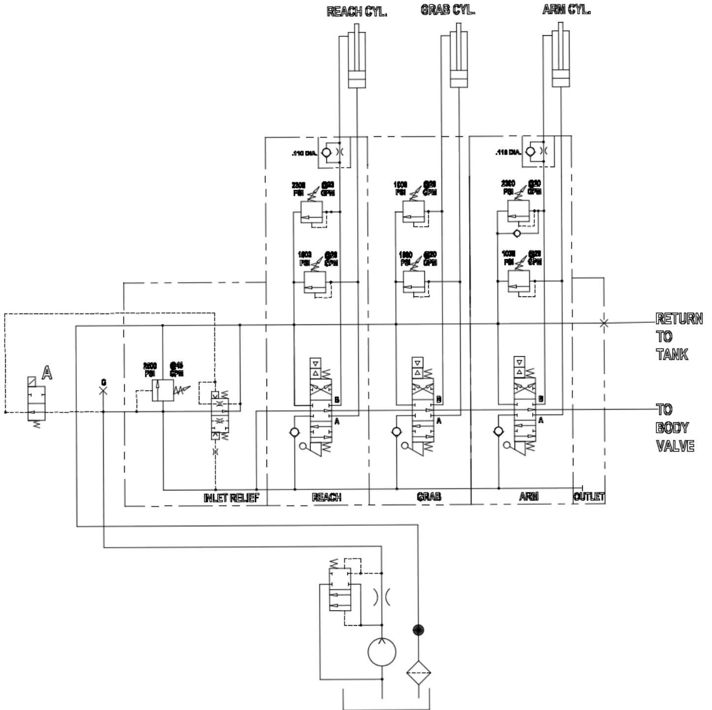
**NOTE:** Solenoid "A" is energized when pump is tuned on.
