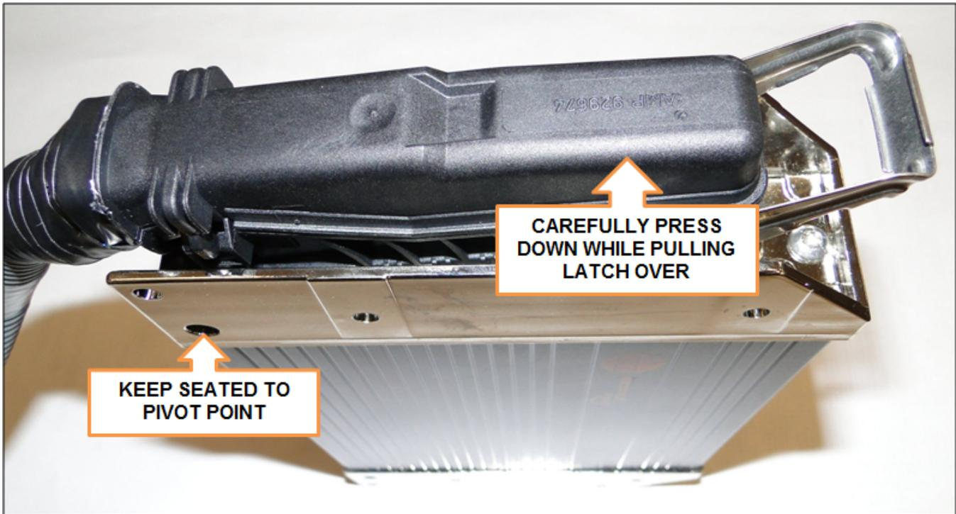
**Figure 48. Slowly Press Down While Keeping Left Cable Connector Pivot Point in Place**
