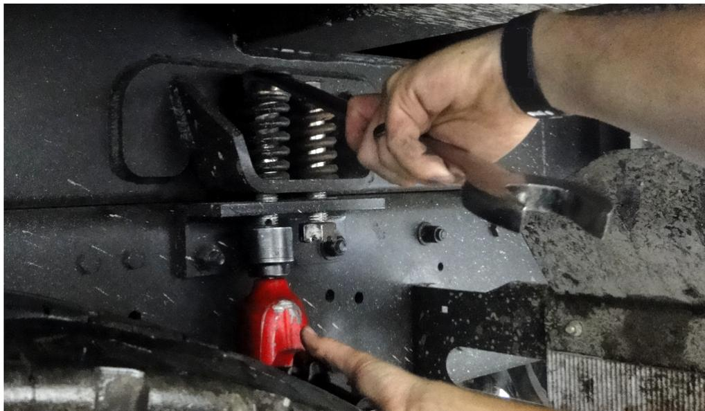
**Figure 28. Removing Bolts and Springs from Chassis Mounting Brackets**
