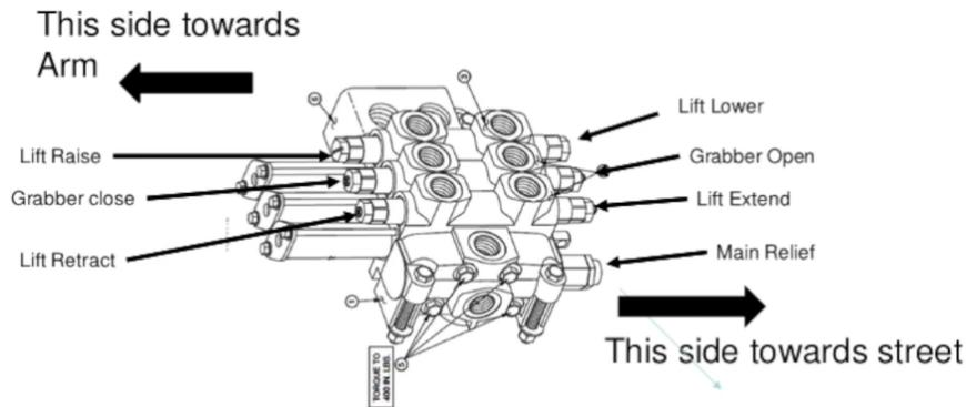
Figure 22. Seven Python Valve Pressure Settings
