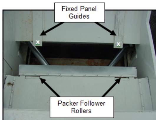
**Figure 39. Packer Pressure Panel Adjustment**
