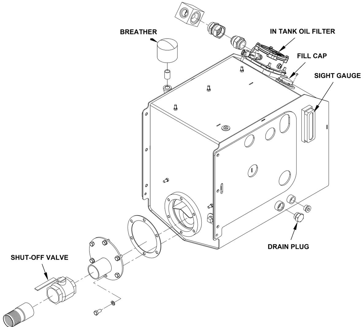
**Figure 40. Hydraulic Oil Tank and Sight Gauge**
