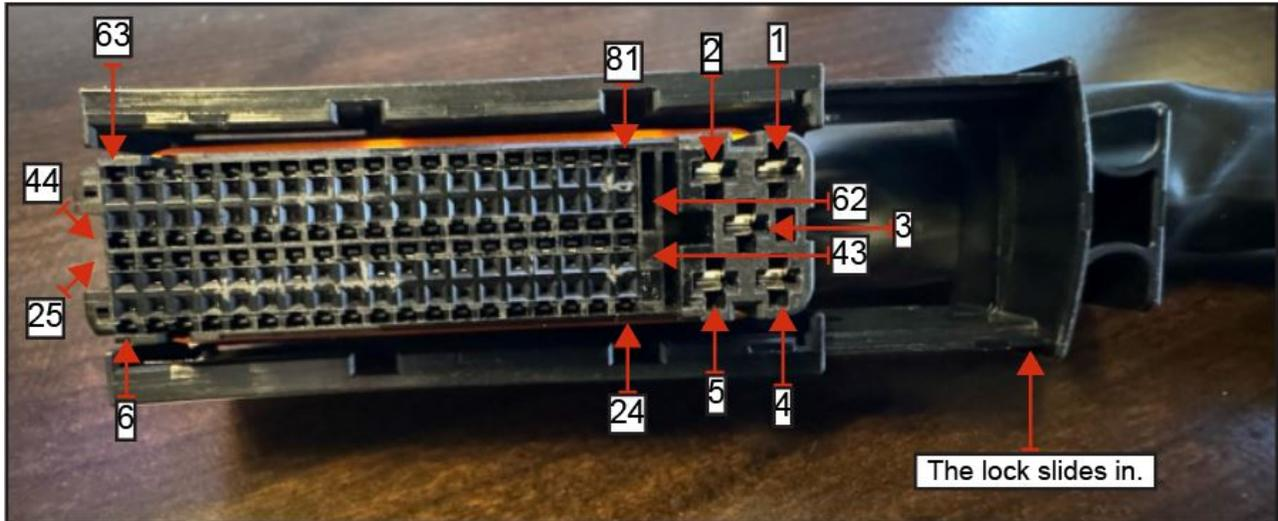
Figure 44. Cortex Cable Connection, Female Pin Positions.
