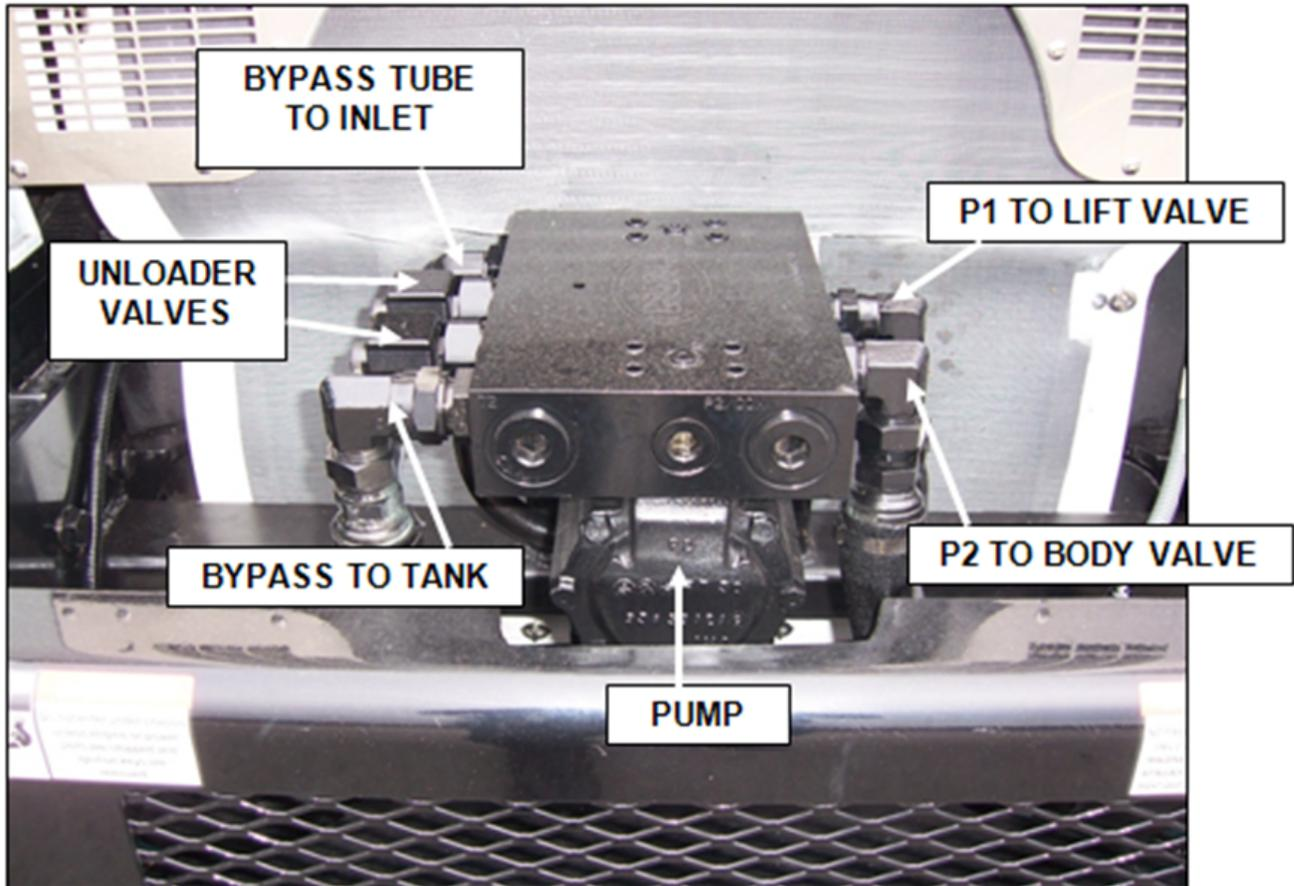
Figure 7. Tandem Vane Pump with Monoblock
