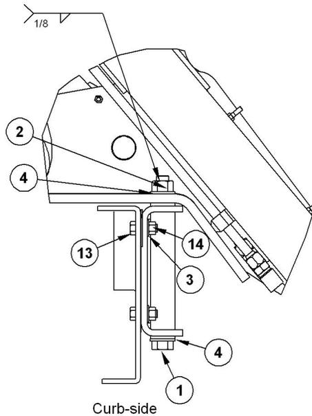
**Figure 14. Lift Mount Bolt Location**
