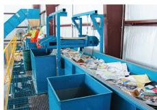
This smaller MRF, located in Bedford County, VA, has a sliderbed sorting line conveyor fed by a combination chain-belt conveyor.
