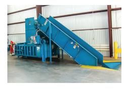
EZ-TRAX sliderbed and steel-belt conveyors are ideal add-ons for baler and compactor-feed applications. They add efficiency to optimize productivity and throughput capacity. This belowground sliderbed is feeding a Gemini® 3560 manual-tie, horizontal baler.
