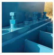
The Galaxy 2R narrow model features an adjustable shear beam that enables you to adjust the shear blades from the exterior of the machine. (Optional on 2R15ON and 2R19ON)
