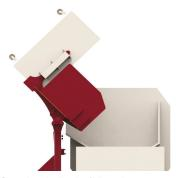
Container is tilted a full 45 degrees past vertical, assuring complete cleanout.
