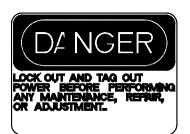
Never enter any part of the compactor unless the power is off and the compactor is locked-out and tagged out in accordance with OSHA requirements.
