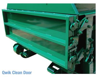
The Qwik Clean® door on the packer end makes cleaning out behind the ram-in-cylinder area a snap. The door has miniature hinges, a door seal, and a ratchet binder. Also, featured is the RamJet® rear-feed-doghouse door option.
