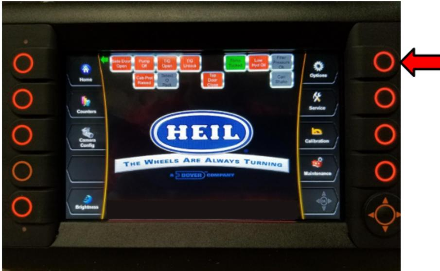
6. To turn the cameras back on, press and hold the top left button on the display for 5 seconds OR cycle the power to the display. See the image below.
