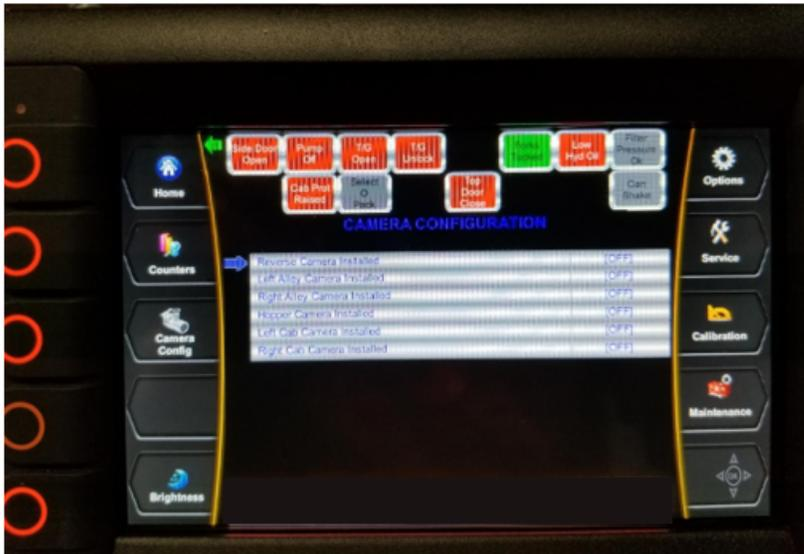
4. Cycle the power to the display and the cameras will be correctly configured.
