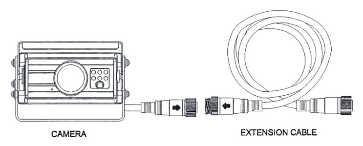
NOTE: Wrap the whole cable connection from one end to another end with Weather-Sealer Strip (NOT SUPPLIED) to ensure adequate insulation against water.
