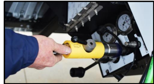
Figure 68. Type 1 Fueling Nozzle
