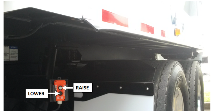
Figure 50. Typical Service Hoist Controls Location
