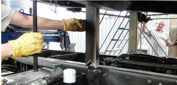
Figure 55. Release and Lower Factory Body Props
