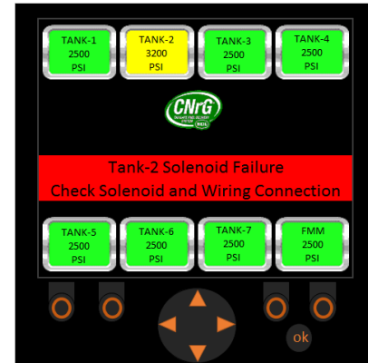
Figure 102. Display Screenshot: Tank 2 Solenoid Failure
