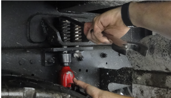
Figure 53. Removing Bolts and Springs from Chassis Mounting Brackets
