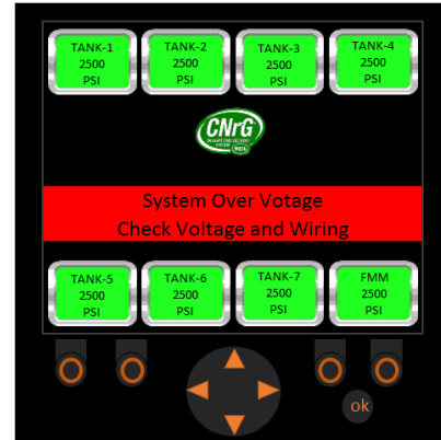
Figure 110. Display Screenshot: System Over Voltage
