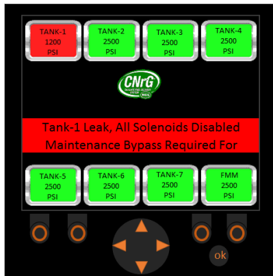
Figure 99. Tank 1 Leak. Maintenance Bypass Required.
