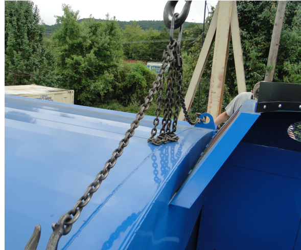
Figure 54. Front Body Chain Hook Lugs
