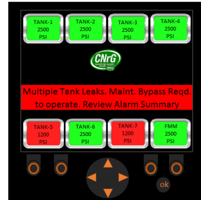
Figure 100. Multiple Tank Leaks. Maintenance Bypass Required.
