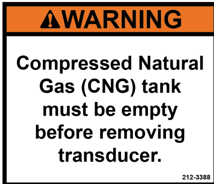
Figure 85. Warning, CNrG Solenoid System, CNG tank empty before removing transducer, PN 212-3388
