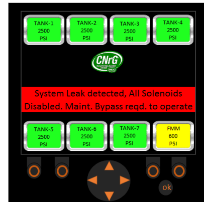
Figure 101. System Leak. Maintenance Bypass Required.
