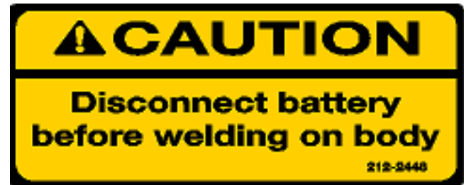
Figure 19. Caution; Disconnect Battery Before Welding, PN 212-2448
