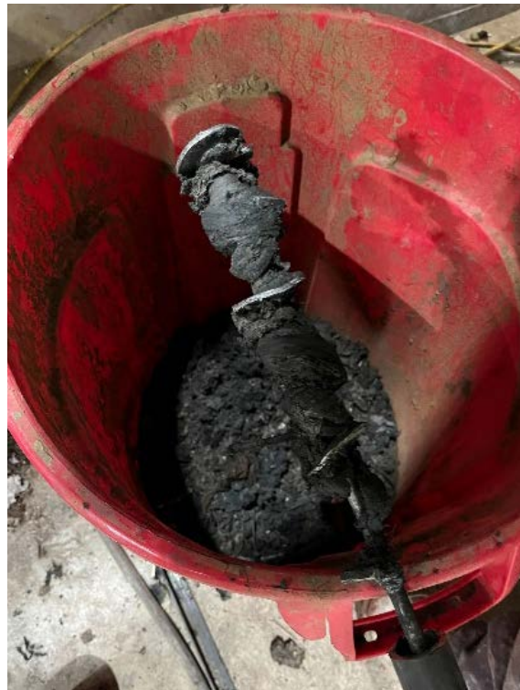
Figure 107. Auger-Type Tool After Removing Waste Material (cloths, plastic bags, and ropes accumulated in the chain canals)
