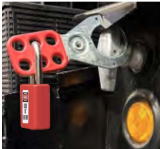
Figure 47. . Chassis Battery Disconnect Switch
