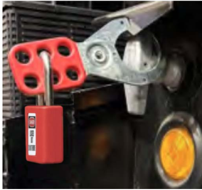
Figure 43. Chassis Battery Disconnect Switch
