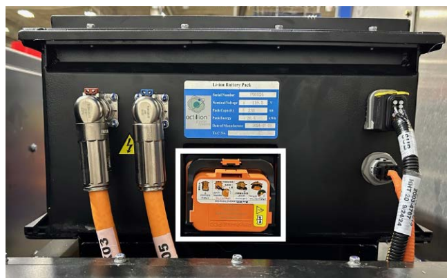
Figure 42. Main System Disconnect (MSD)
