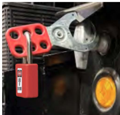
Figure 25. Chassis Battery Disconnect Switch
