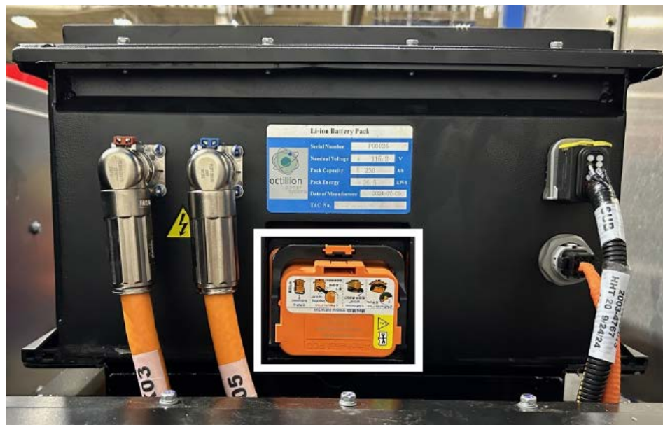
Figure 29. Main System Disconnect (MSD)
