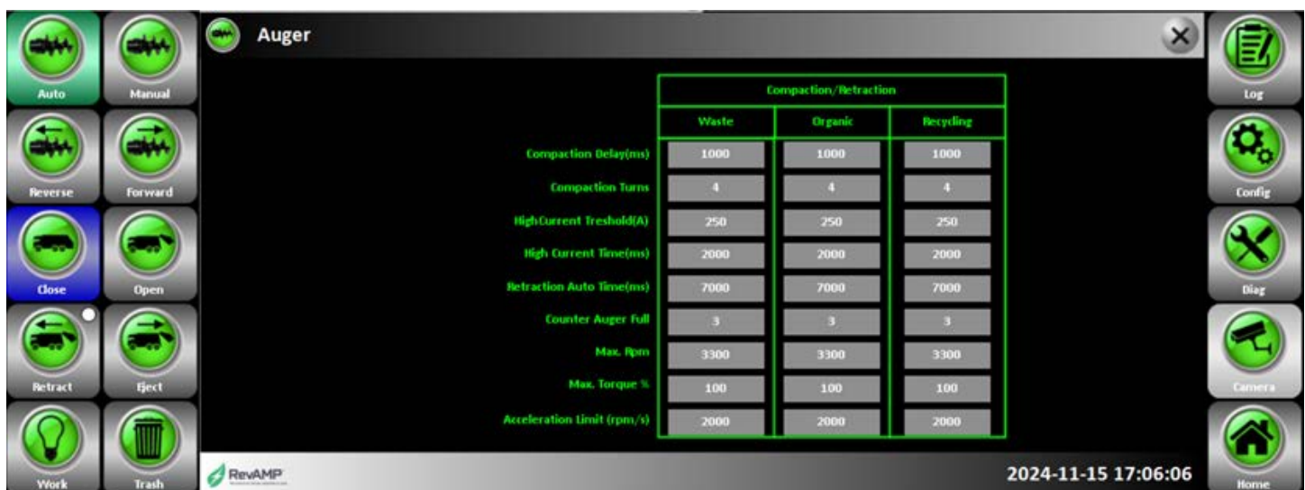
Figure 123. Auger Configuration Screen
