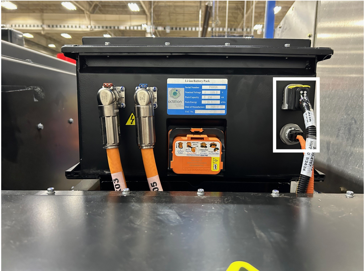
Figure 35. Communications Power Connectors (White Outlined Box)
