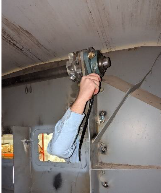
Figure 59. Lubricate the Two Bearings Through the Access Window
