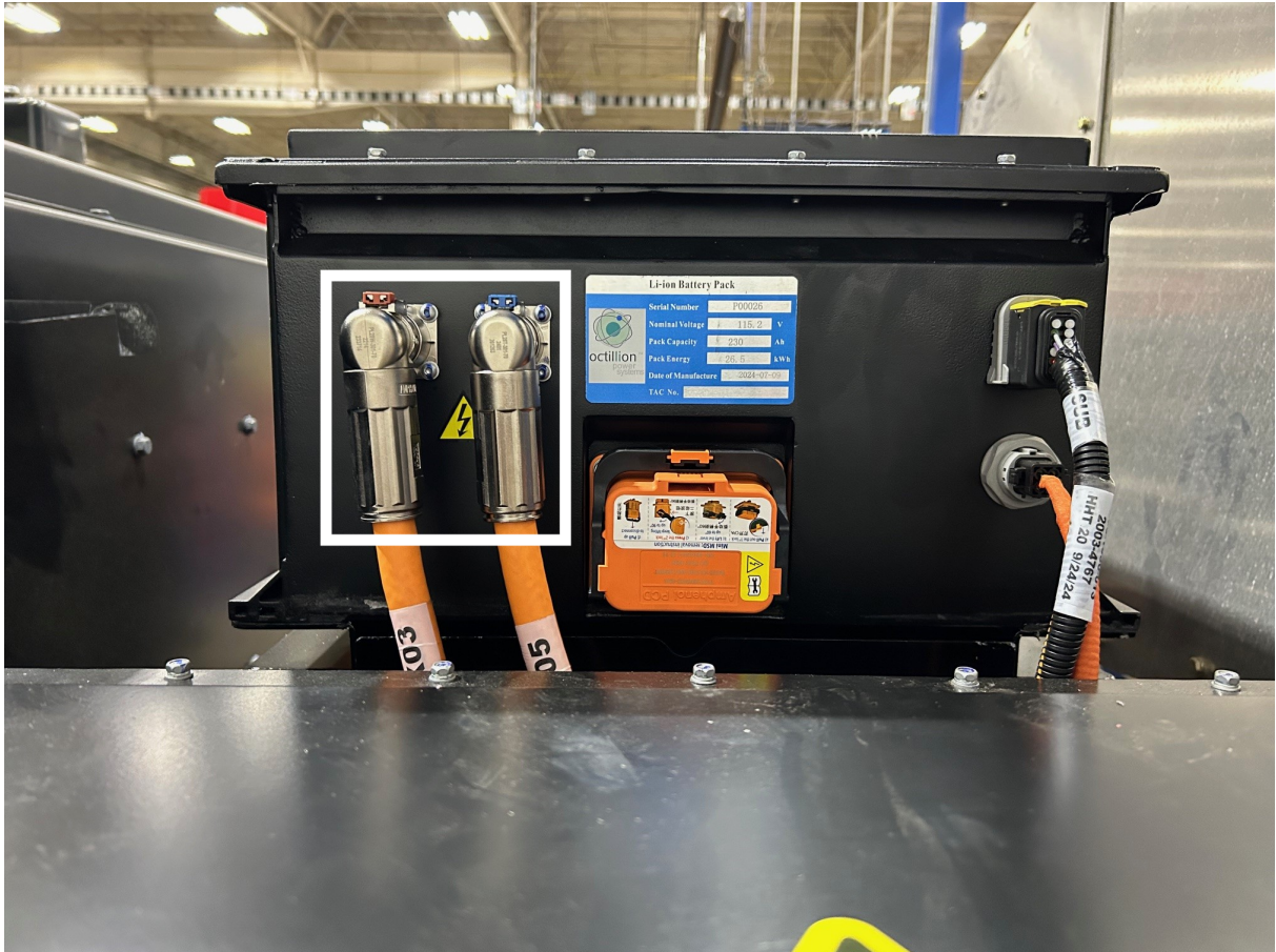
Figure 34. Body Battery Power Connectors (White Outlined Box)
