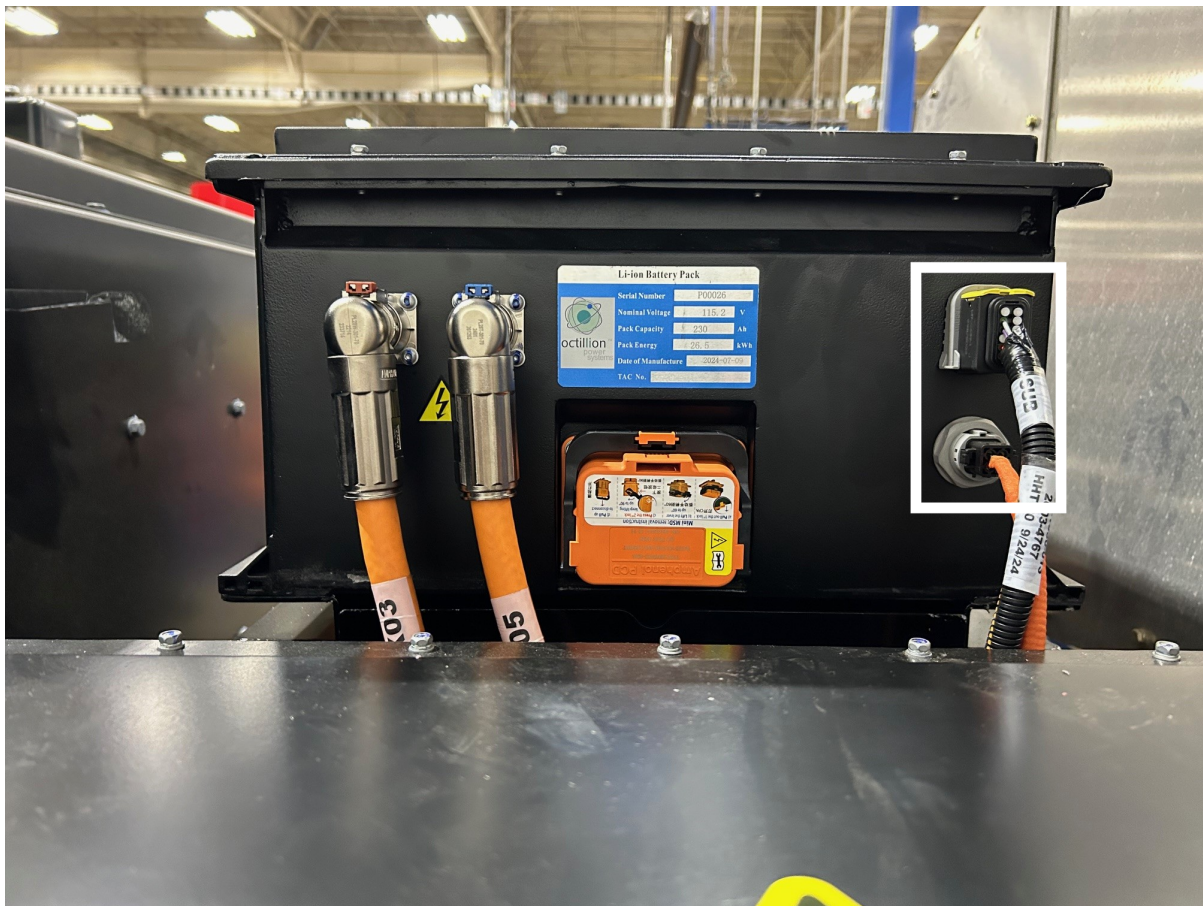
Figure 39. Communications Power Connectors (White Outlined Box)
