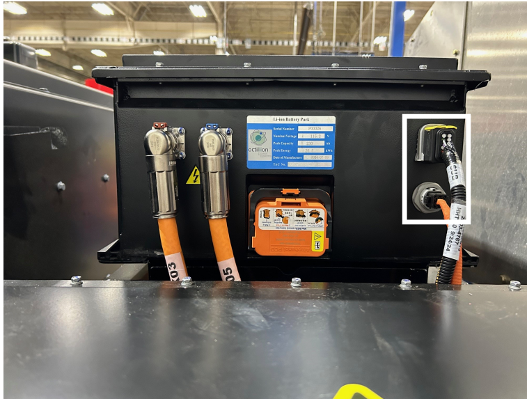
Figure 24. Battery Low Voltage and Heater Power Connectors (White Outlined Box)
