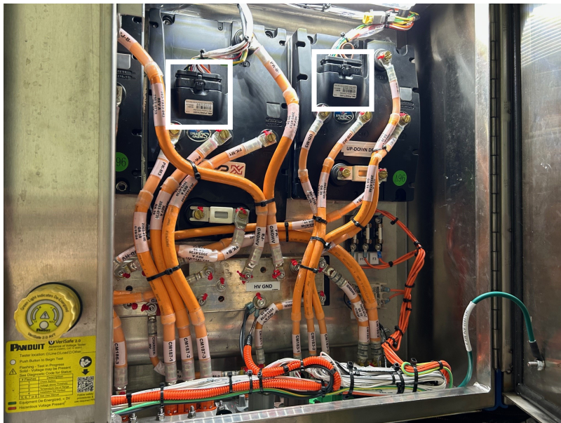
Figure 27. Body High Voltage Electrical Cabinet Panel 2 (2 Locations)
