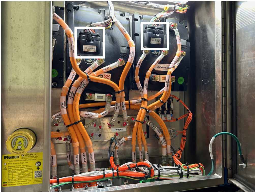
Figure 33. Body High Voltage Electrical Cabinet Panel 2 (2 Locations)
