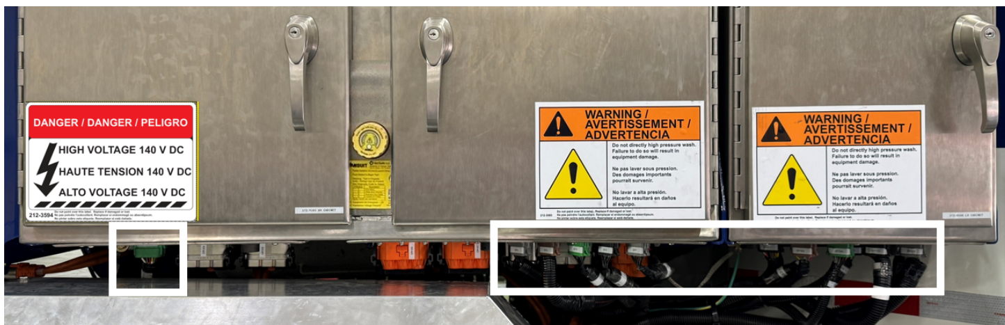
Figure 30. Locations of the Low Voltage Connectors (White Outlined Boxes)
