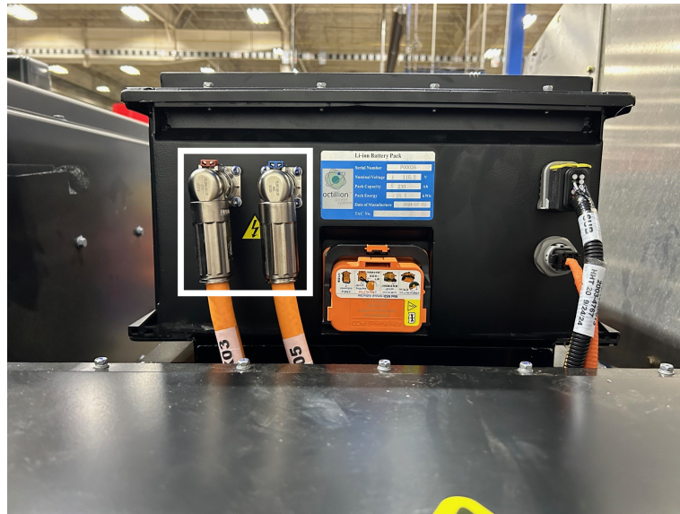
Figure 25. Battery High Voltage Power Connectors (White Outlined Box)
