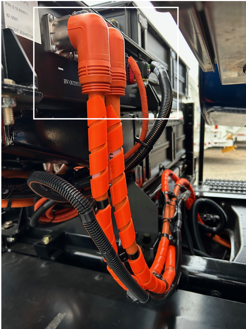
Figure 31. Location of the Battery Management System (BMS) Connectors (White Outlined Box)
