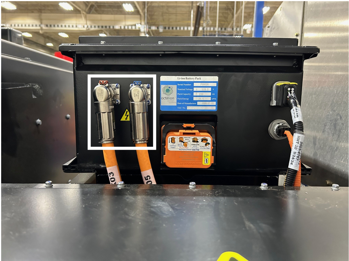
Figure 38. Battery Power Connectors (White Outlined Box)
