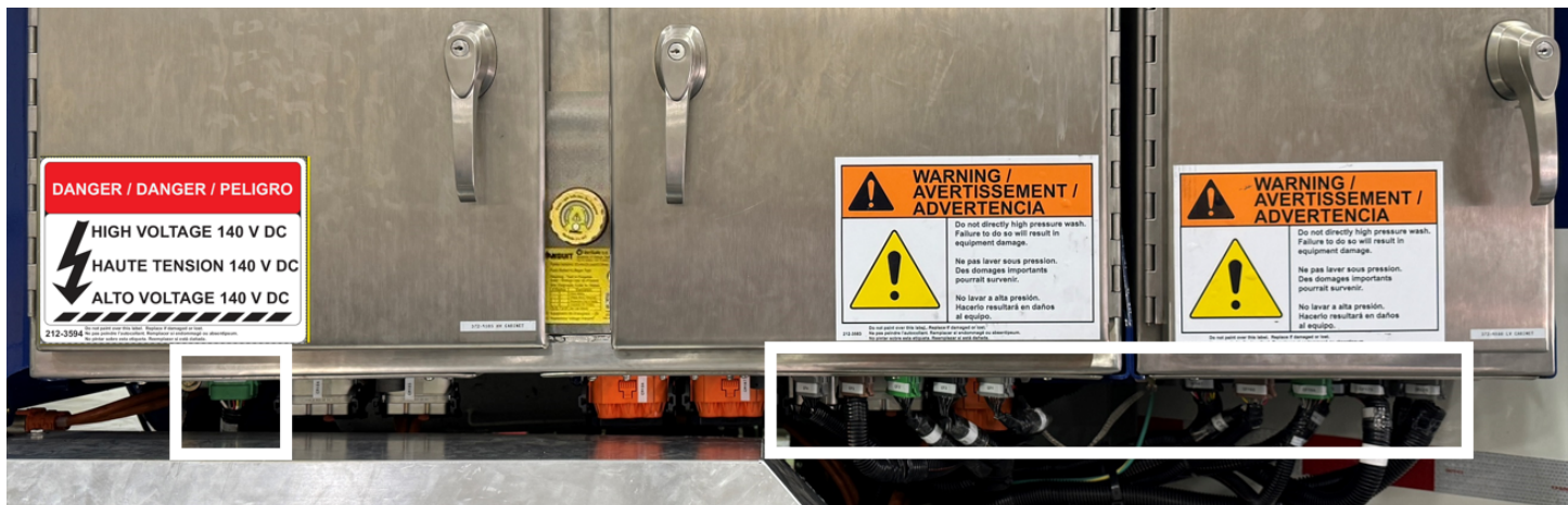
Figure 21. Locations of the Low Voltage Connectors (White Outlined Boxes)
