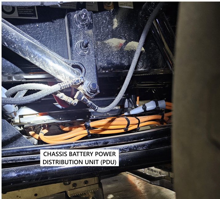
Figure 46. PDU Location on a Peterbilt EV Chassis Viewed from the Street Side Wheel Well Beneath the Cab
