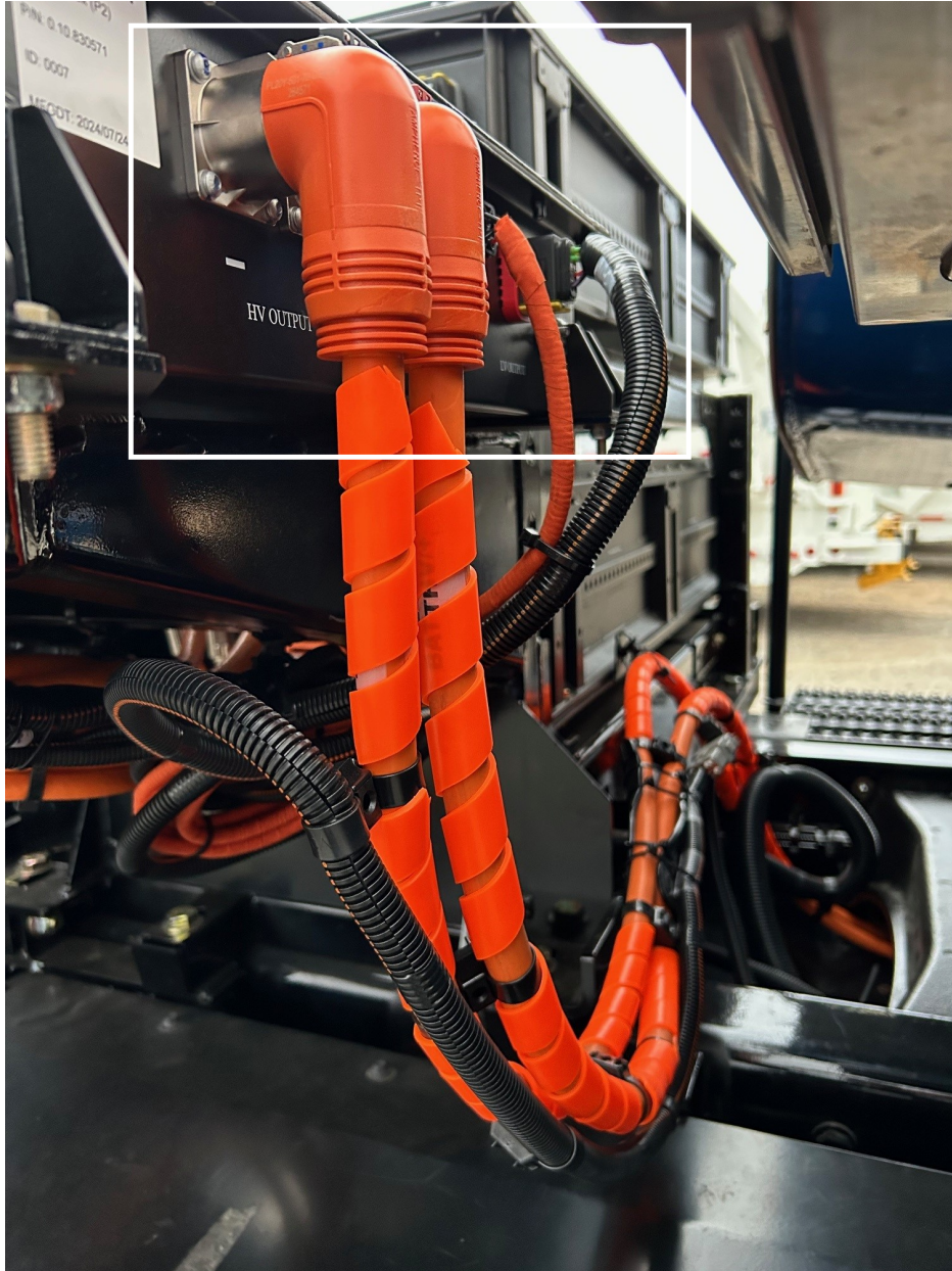
Figure 28. Location of the Battery Management System (BMS) Connectors (White Outlined Box)
