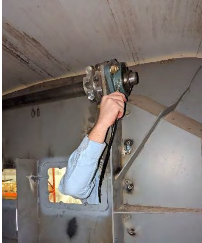
Figure 61. Lubricate the Two Bearings Through the Access Window
