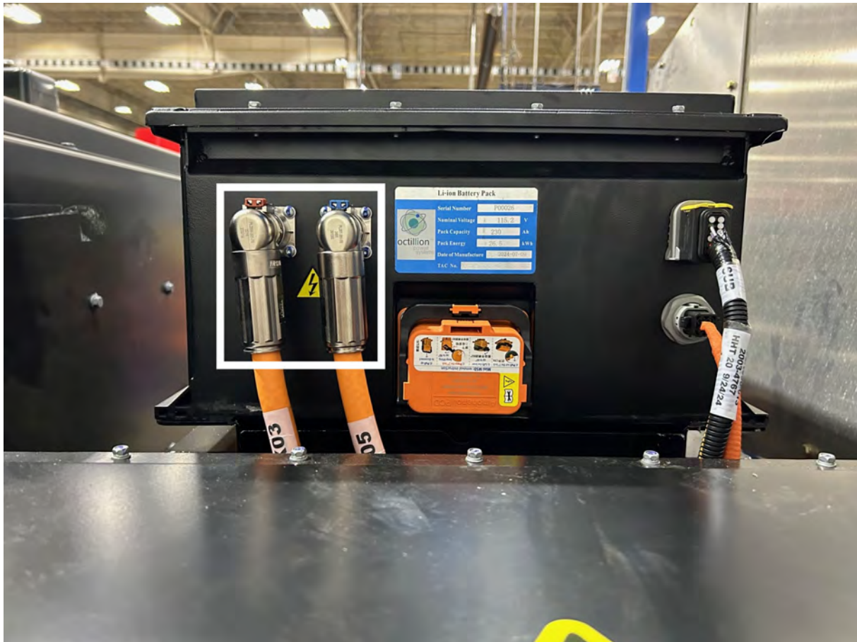
Figure 40. Battery Power Connectors (White Outlined Box)
