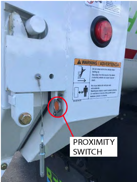
Figure 72. Proximity Switch Location
