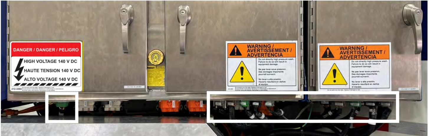
Figure 23. Locations of the Low Voltage Connectors (White Outlined Boxes)
