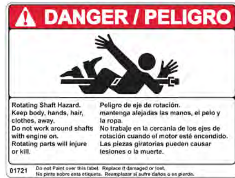
Figure 20. Danger Rotating Shaft, PN 01721
