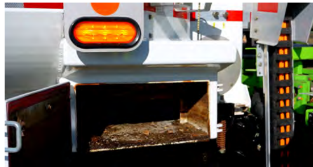
Figure 102. Curb Side Sump Door Open
