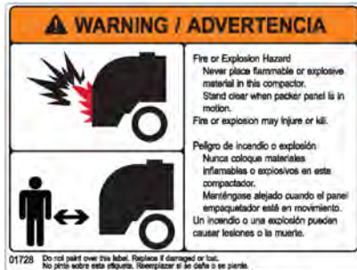
Figure 21. Fire or Explosion , PN 01728
