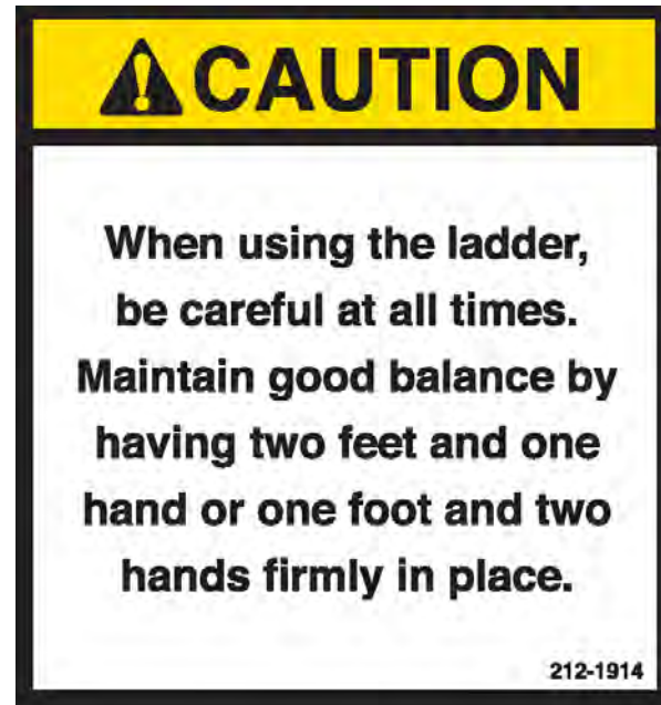
Figure 30. Caution When Using the Ladder, PN 212-1914
