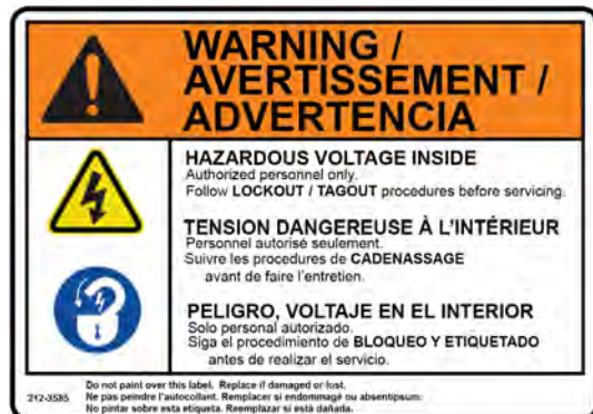
Figure 40. Warning: Hazardous Voltage Inside, PN 212-3585
