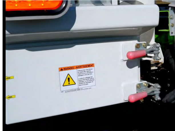
Figure 101. Sump Door Closed
