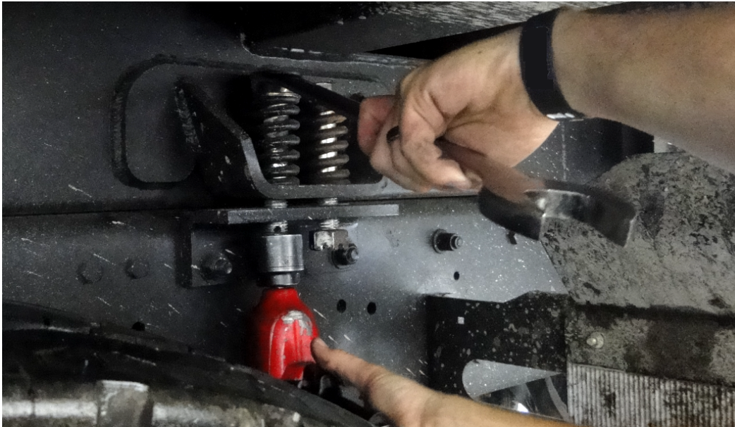
Figure 41. Removing Bolts and Springs from Chassis Mounting Brackets
