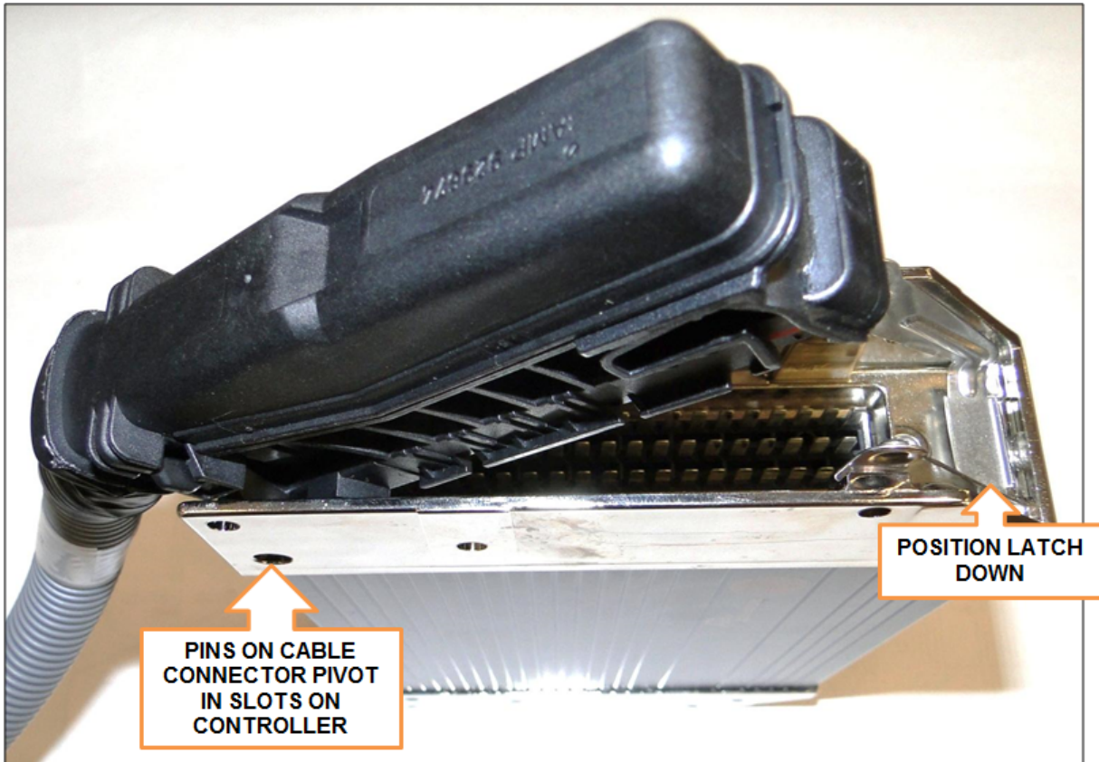
Figure 68. Cable Connector Pivoting on Controller
