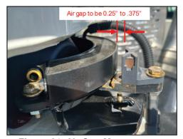
Figure 84. Air Gap Measurement
