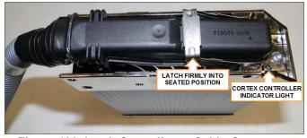
Figure 106. Latch Controller to Cable Connector
