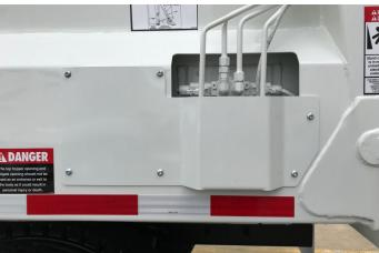
Figure 97. Tailgate Valve with Cover
