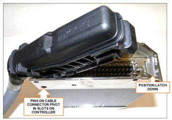
Figure 104. Cable Connector Pivoting on Controller
