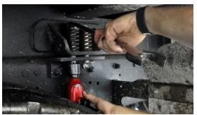
Figure 61. Removing Bolts and Springs from Chassis Mounting Brackets
