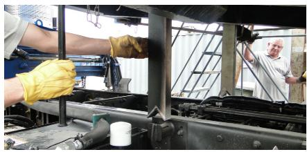
Figure 65. Release and Lower Factory Body Props
