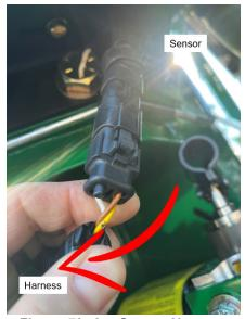
Figure 79. Arc Sensor Harness
