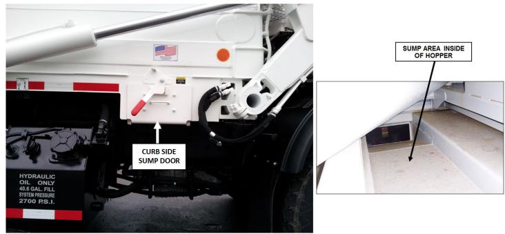
Figure 73. Sump Door and Internal Area
