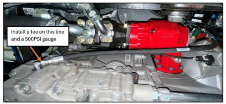
Figure 48. Transmission Pressure Feed to PTO.
