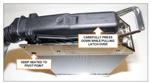
Figure 105. Slowly Press Down While Keeping Left Cable Connector Pivot Point in Place
