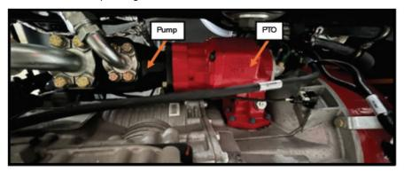
Figure 44. Direct Mount Pump.
