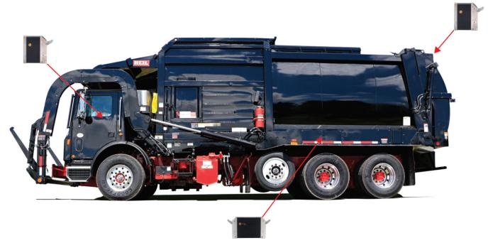
Figure 100. Mobile Controller Locations
