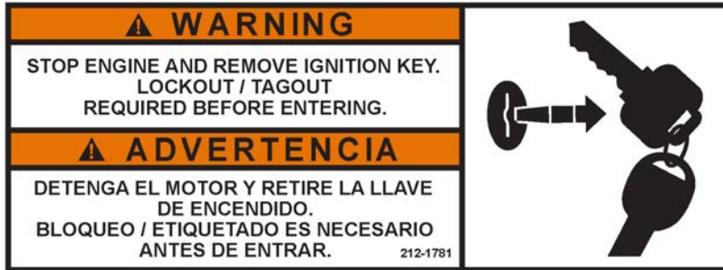
Figure 8. Warning: Lock-out / Tag-out, PN 212-1781
