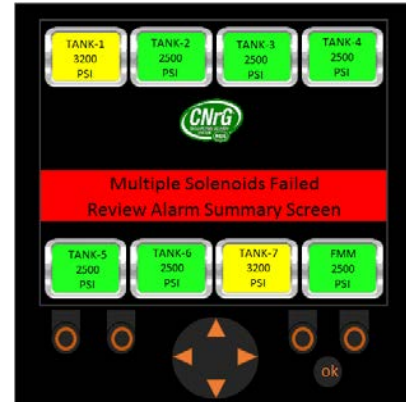
Figure 96. Display Screenshot: Multiple Solenoids Failed
