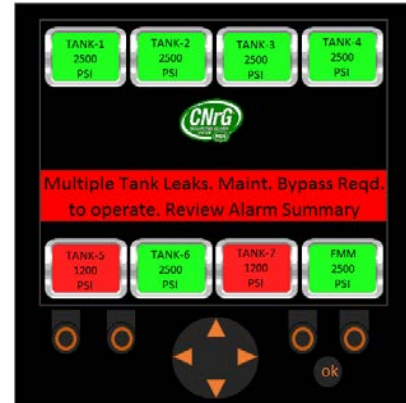
Figure 93. Multiple Tank Leaks. Maintenance Bypass Required.
