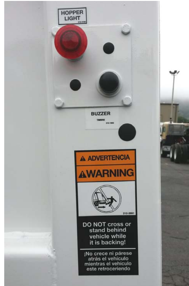
Figure 49. Buzzer and Hopper Light Switch Location
