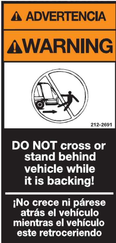
Figure 16. Warning: Do not cross/stand behind, PN 212-2691
