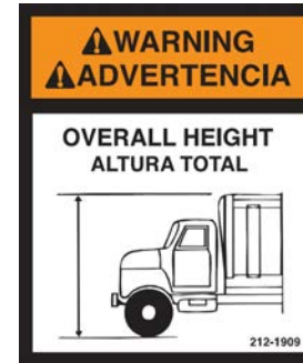
Figure 20. Warning: Overall height, PN 212-1909
