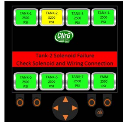
Figure 95. Display Screenshot: Tank 2 Solenoid Failure
