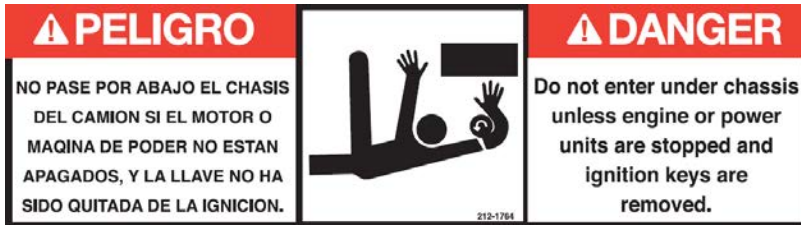
Figure 10. Danger: Do not enter under, PN 212-1764
