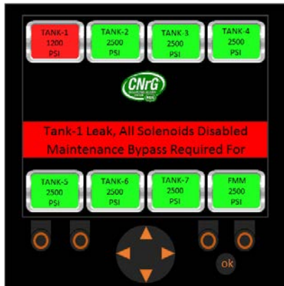
Figure 92. Tank 1 Leak. Maintenance Bypass Required.
