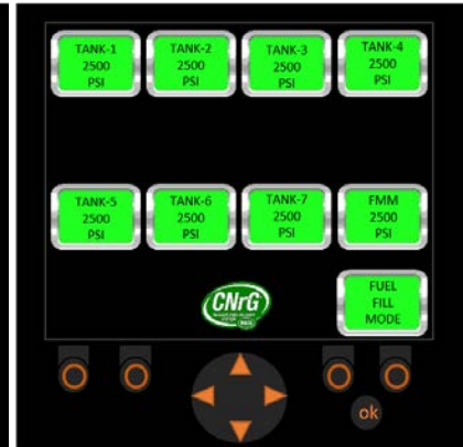
Figure 106. Display Screenshot: Fuel Fill Mode ON
