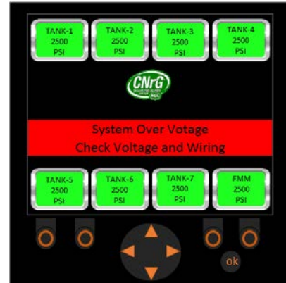
Figure 103. Display Screenshot: System Over Voltage
