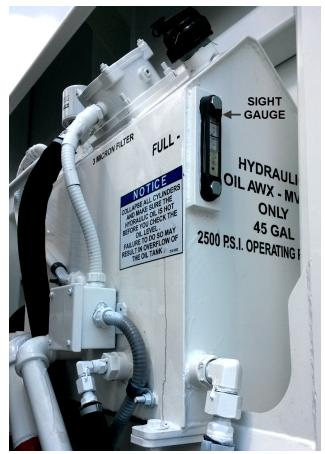
Figure 56. Hydraulic Oil Tank with Sight Gauge
