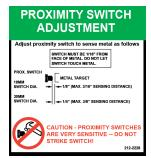
Figure 12. Proximity Switch, Adjustment, PN 212-2228
