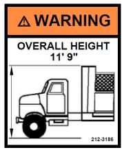
Figure 21. In-Cab, Overall Height, 11'9", PN 212-3186
