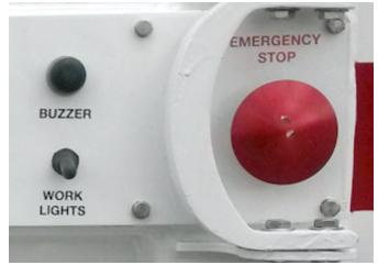
Figure 59. Outside Tailgate Controls (Both Sides)
