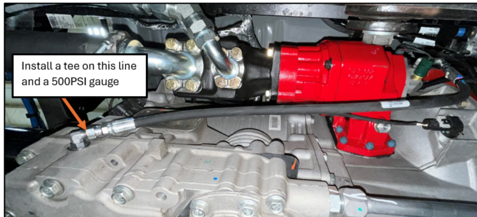
Figure 21. Transmission Pressure Feed to PTO
