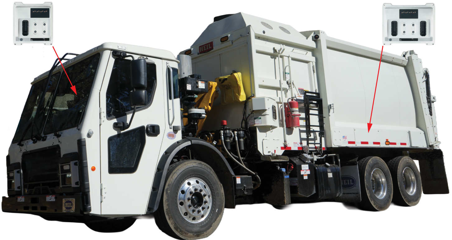
Figure 130. Mobile Controller Locations
