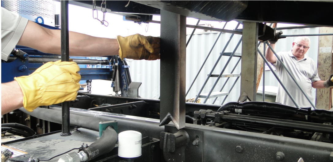
Figure 58. Release and Lower Factory Body Props
