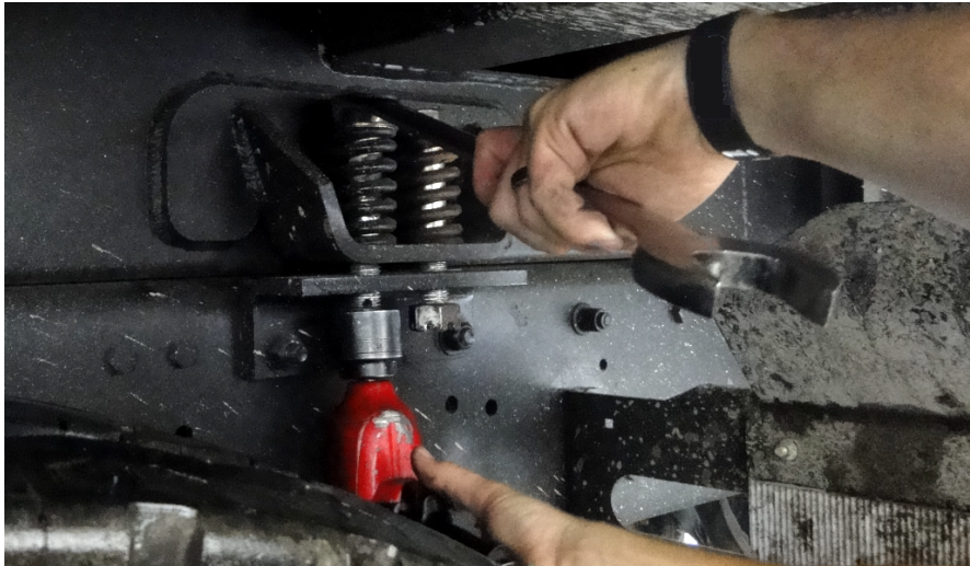
Figure 56. Removing Bolts and Springs from Chassis Mounting Brackets
