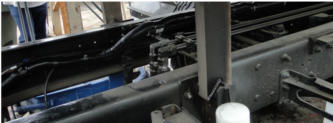
Figure 59. Release and Lower Factory Body Props
