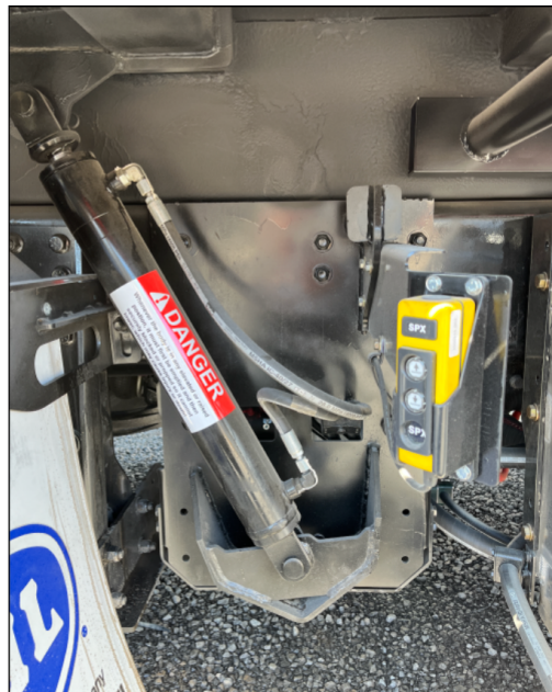
Figure 48. Service Hoist Controller
