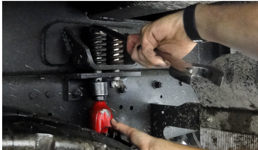
Figure 54. Removing Bolts and Springs from Chassis Mounting Brackets
