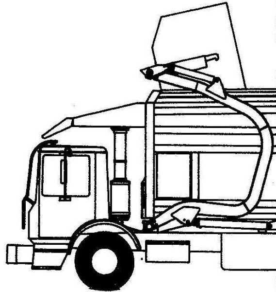
Figure 106. Dump Container Into Hopper
