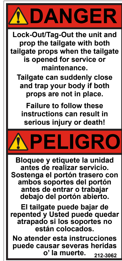
Figure 37. Danger: Tailgate Props Operation, PN 212-3062
