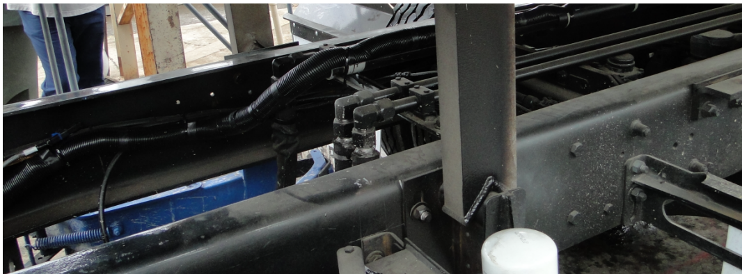
Figure 77. Release and Lower Factory Body Props
