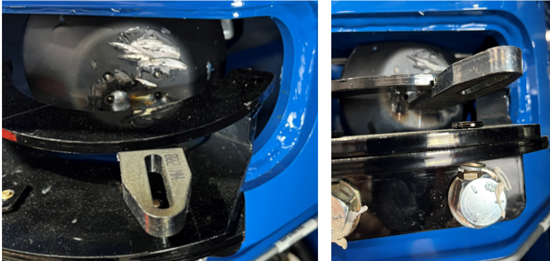
Figure 109. Magnet Holder Location on Cylinder Rod Eye
