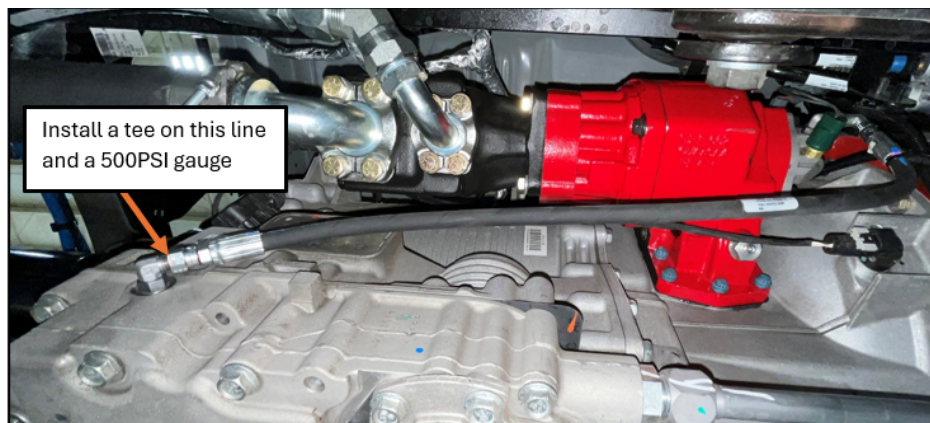
Figure 59. Transmission Pressure Feed To Pto
