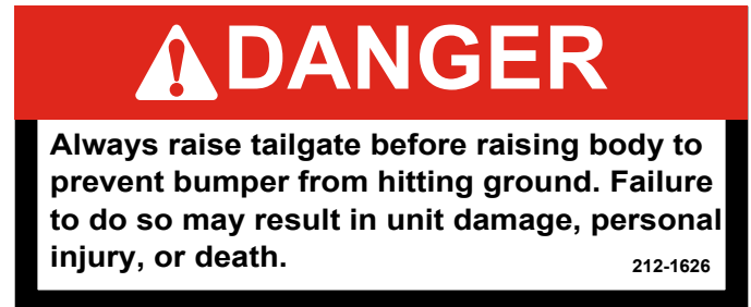
Figure 18. Danger: Raise Tailgate Before Raising Body, PN 212-1626
